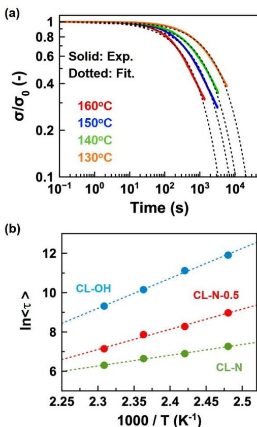
Figure S16. (a) Stress relaxation curves for CL-N-0.5. In the Y-axis, the stress ( $\sigma$ ) was normalized by the initial stress ( $\sigma_0$ ). The dotted curves indicate the fitting curves based on the KWW function (see main text). (b) Temperature dependence of  $\langle \tau \rangle$  for CL-N, CL-OH, and CL-N-0.5. The dotted line indicates the approximate straight line between the points.
