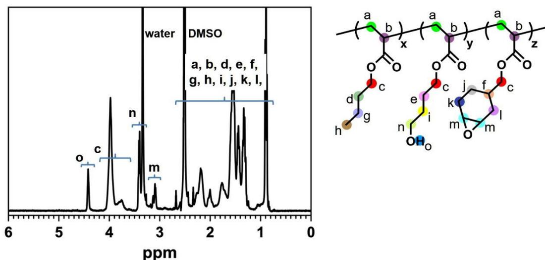
Figure S4.  $^1\text{H-NMR}$  spectrum of P-OH in  $\text{DMSO-}d_6$ .
