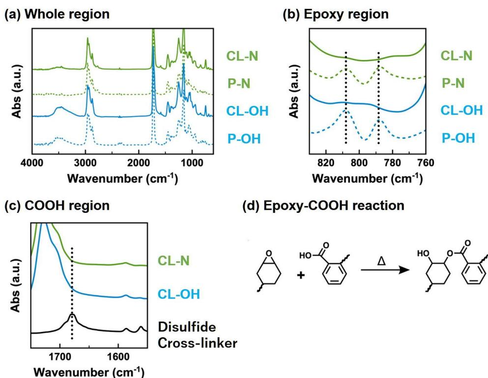
Figure S7. FT-IR spectra for the precursor polymers and cross-linked samples at (a) whole region, (b) epoxy region, and (c) COOH region. The dotted lines in (b) and (c) indicate the signals from epoxy and the signal from COOH group, respectively, according to the literature (refs #56 and 57 in the main text). Schematic of the reaction between COOH and epoxy is shown in (d).
