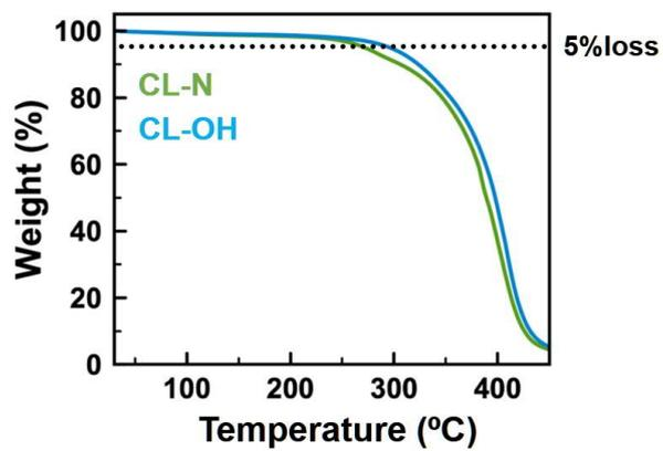
Figure S9. TGA thermograms for the cross-linked samples.
