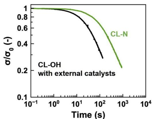
Figure S11. Stress relaxation curve for CL-OH with external amine catalysts, where the data for CL-N is also shown for comparison. In the Y-axis, the stress ( $\sigma$ ) was normalized by the initial stress ( $\sigma_0$ ). The data were taken at 160 °C.
