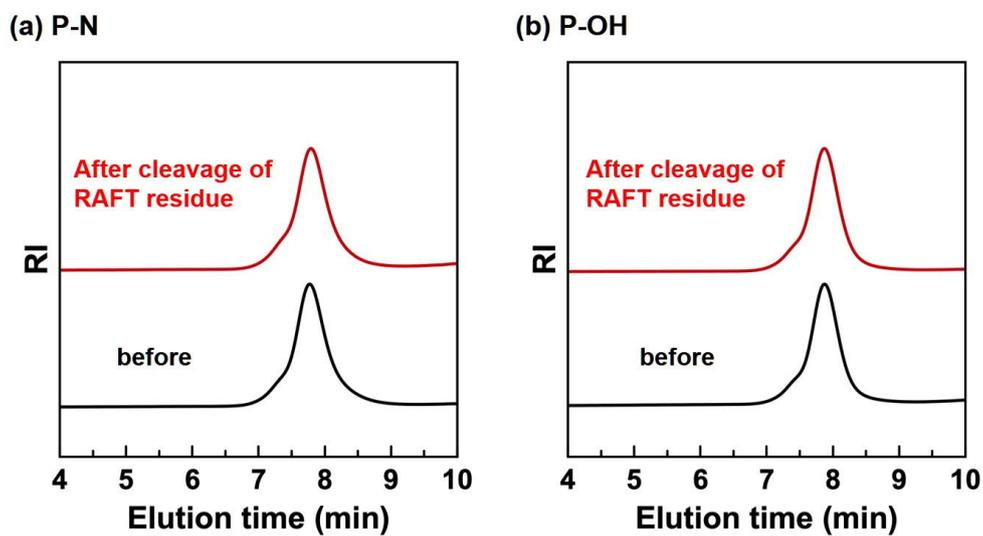
Figure S5. SEC curves for P-N and P-OH before and after cleavage of the end RAFT residue.
