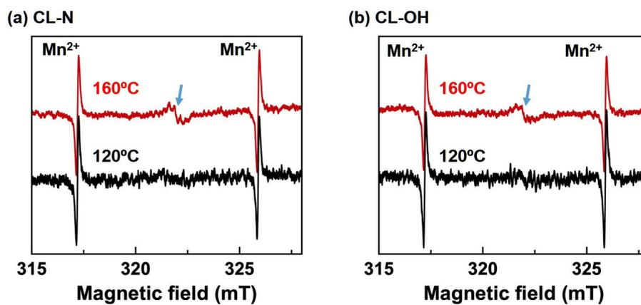
Figure S17. ESR spectra measured at 120 and 160 °C for CL-N and CL-OH. The arrows represent the signal from sulfide radical, and the distinct outside signals were from  $Mn^{2+}$  used for the magnetic field calibration.
