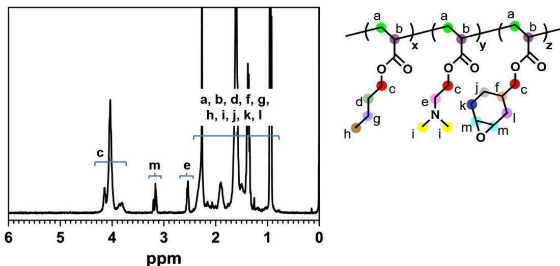
Figure S3.  $^1\text{H-NMR}$  spectrum of P-N in  $\text{CDCl}_3$ .
