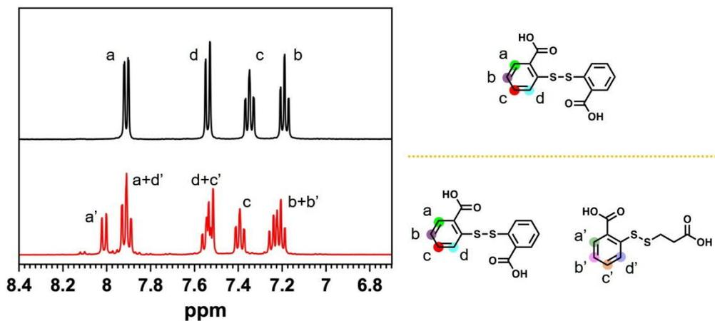
Figure S2. <sup>1</sup>H-NMR spectra for starting DBA (top) and the residue after stirring in the presence of tertiary amines (bottom). H<sub>x</sub> with alphabet (x) in the spectra corresponds to the protons with the same alphabet in the chemical structures. Note that the signal position was slightly different from that in Figure S1, which is due to the presence of amines that should have some interaction with COOH group.
