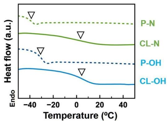
Figure S8. DSC thermograms for the samples before and after cross-linking reaction. The data were obtained in the second heating. The inverse triangles represent  $T_g$ .
