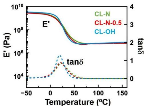
Figure S15. Temperature-sweep rheology data for CL-N-0.5, where the data of CL-N and CL-OH are shown for comparison.
