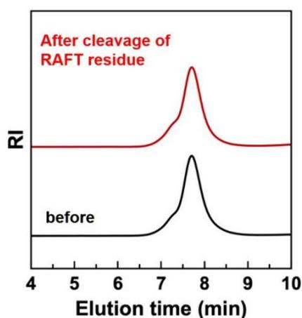
Figure S14. SEC curves for P-N-0.5 before and after cleavage of the end RAFT residue.
