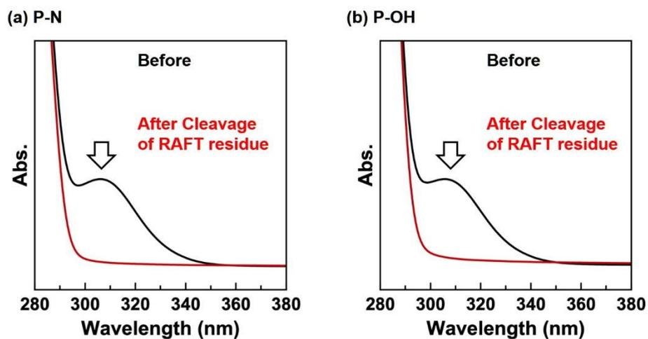
Figure S6. UV-vis spectra for P-N and P-OH before and after cleavage of the RAFT residue. The arrows indicate the characteristic absorption signal from the trithiocarbonate end group.
