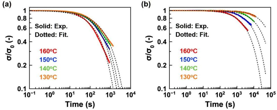
Figure S12. Stress relaxation curves for (a) CL-N and (b) CL-OH at various temperatures. In the Y-axis, the stress ( $\sigma$ ) was normalized by the initial stress ( $\sigma_0$ ). The dotted curves indicate the fitting curves based on the KWW function (see main text).
