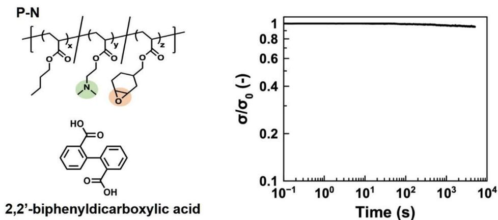
Figure S10. Stress relaxation data at 160 °C for the control sample without disulfide bonds.
