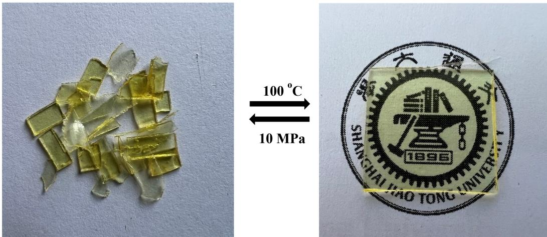
**Figure S8** Photographs of P(BA<sub>55</sub>-POSS<sub>15</sub>-HUB<sub>30</sub>) for the reprocessing test
