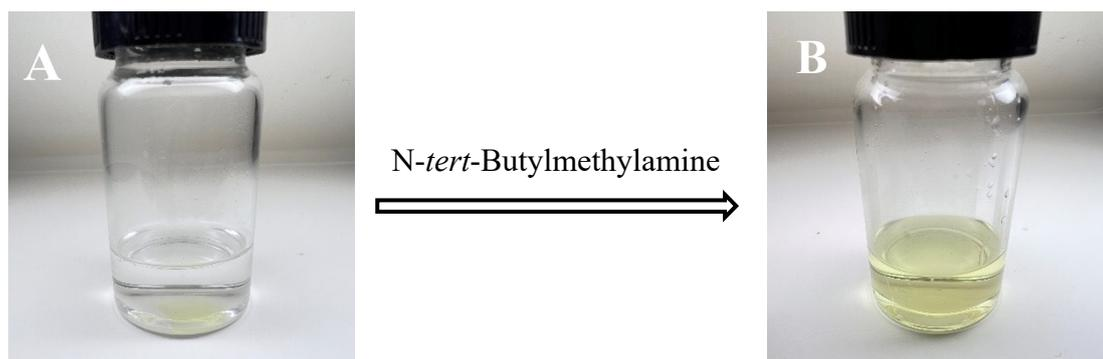
**Figure S5** Photographs of solubility tests for P(BA<sub>75</sub>-POSS<sub>15</sub>-HUB<sub>10</sub>) network: A) swollen with 1,4-dioxane for 12 hours; B) held at room temperature for 12 hours after *N-tert*-butylmethylamine was added
