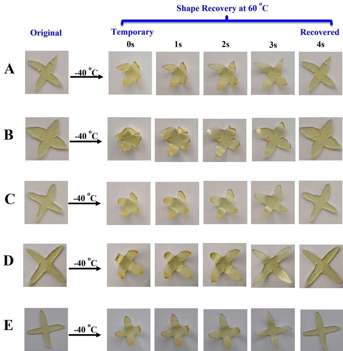
**Figure S9** Shape recovery processes of A: P(BA<sub>75</sub>-POSS<sub>15</sub>-HUB<sub>10</sub>), B: P(BA<sub>65</sub>-POSS<sub>15</sub>-HUB<sub>20</sub>), C: P(BA<sub>55</sub>-POSS<sub>15</sub>-HUB<sub>30</sub>), D: P(BA<sub>70</sub>-POSS<sub>10</sub>-HUB<sub>20</sub>) and E: P(BA<sub>60</sub>-POSS<sub>20</sub>-HUB<sub>20</sub>) for the their temporary shapes at 60 °C
