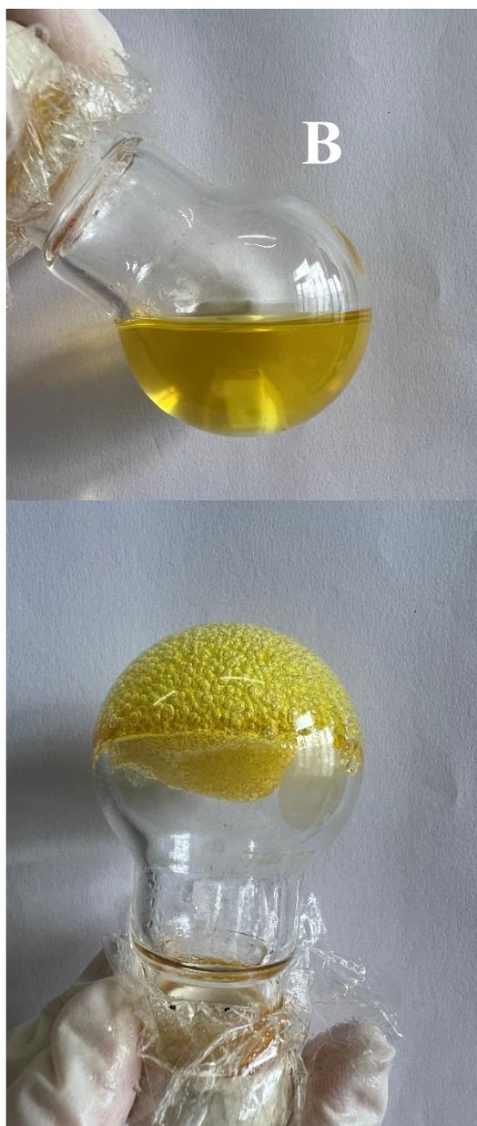
**Figure S4** Photographs for P(BA<sub>65</sub>-POSS<sub>15</sub>-BMEA<sub>20</sub>) copolymer: A) the solution of 1,4-dioxane at the concentration of  $1 \text{ g} \times \text{mL}^{-1}$ ; B) the mixture after 1,2-bis(tert-butyl)ethylenediamine (50 mol% with respect to the quantity of BMEA) was added and reacted at 80 °C
