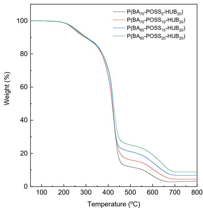
**Figure S3** TGA curves of P(BA-POSS-BMEA) copolymers in an air atmosphere and at the heating rate of  $20\text{ }^{\circ}\text{C} \times \text{min}^{-1}$
