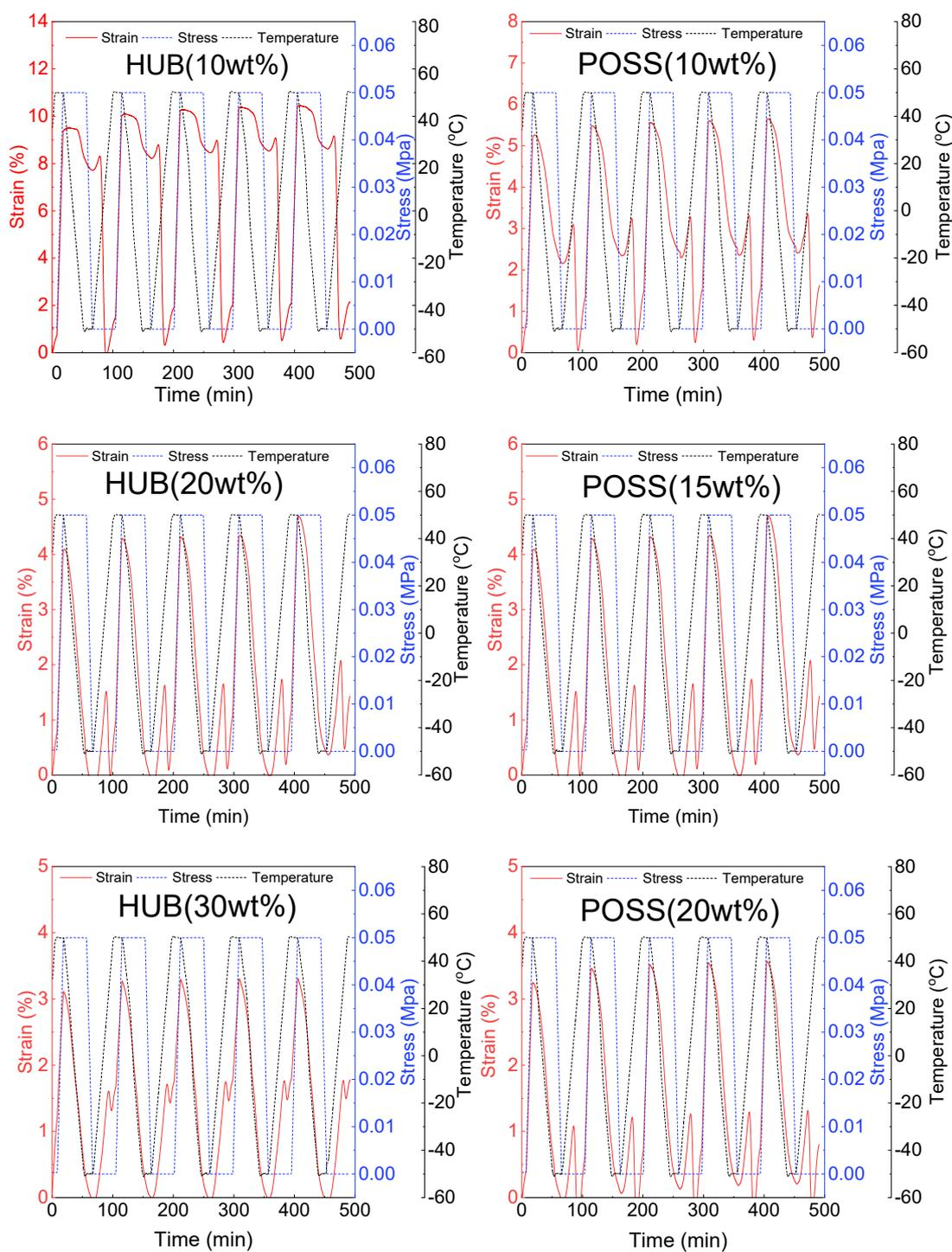
**Figure S10** One-way shape memory cycles curves of P(BA-POSS-HUB) networks:
