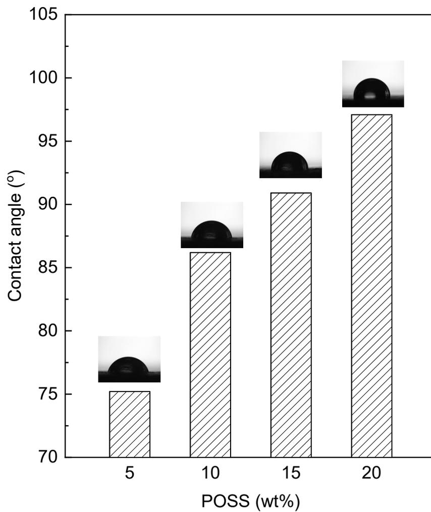
**Figure S6** Plot of water contact angles of P(BA-POSS-HUB) networks as a function of POSS contents
