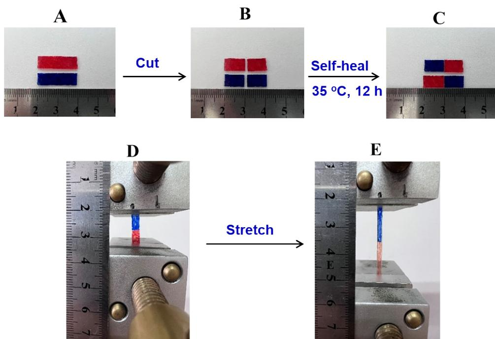
**Figure S7** Photographs of P(BA<sub>75</sub>-POSS<sub>15</sub>-HUB<sub>10</sub>) for self-healing test: A) Two original specimens were colored in red and blue; B) they were cut into four halves; C) two halves with different colors were exchanged and put in contact for self-healing at 35 °C for 12 h; D) the healed specimen was used for stretching; E) the healed specimen can be uniaxially stretched at the elongation of  $\varepsilon = 135\%$  without break
