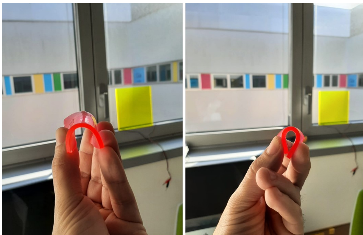
Figure S7. Photographs of a bent LSC device (LSC2_150)
