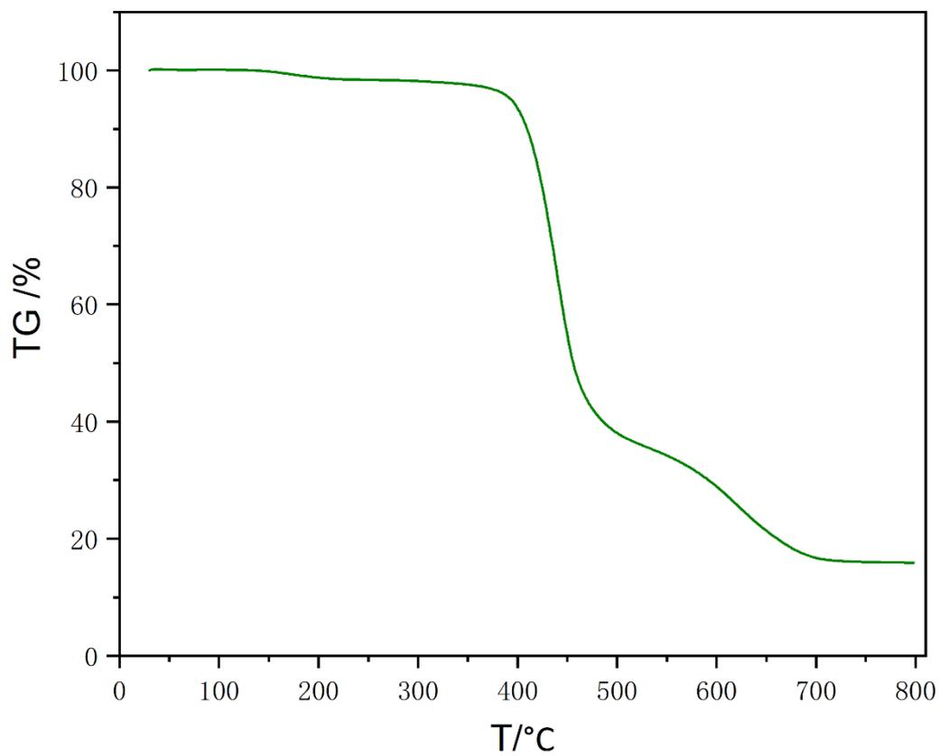
**Figure S12.** Thermogravimetric curve for **P2b** taken at 20 °C/ min to 800°C in N<sub>2</sub>.
