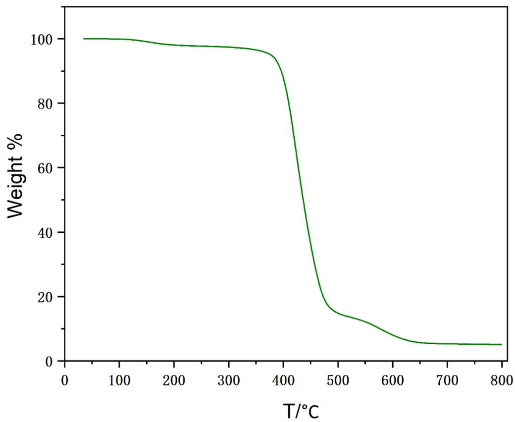
**Figure S14.** Thermogravimetric curve for **P4** taken at 20 °C/ min to 800°C in N<sub>2</sub>.
