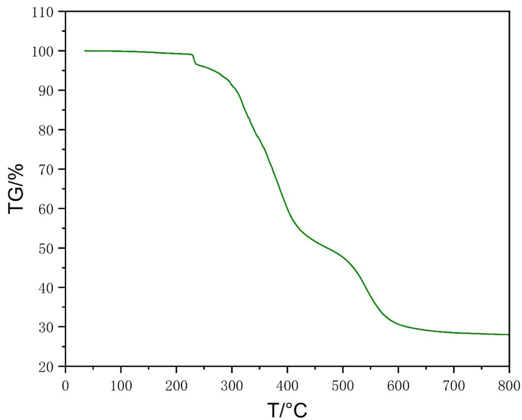
**Figure S13.** Thermogravimetric curve for **P3** taken at 20 °C/ min to 800°C in N<sub>2</sub>.
