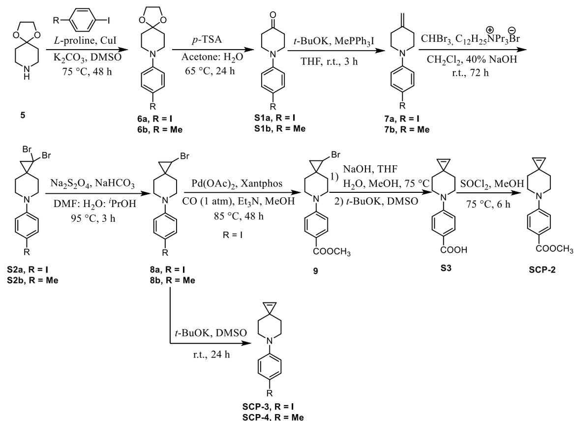
**Scheme S1.** Synthetic route of monomer **SCP-2**, **SCP-3** and **SCP-4**
