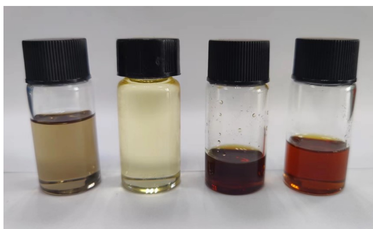
Figure S36. Color of main reactants and products. (a) Cardanol (b) Cardanol diol (c) r-PET diol (d) r-PET PUA
