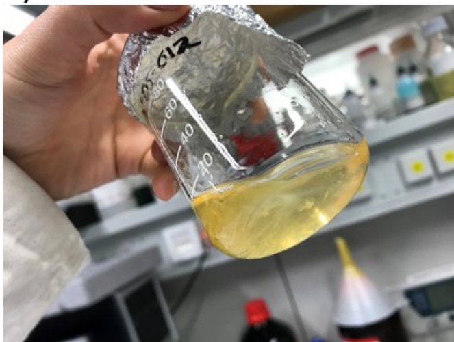
Figure SI 16. Representative images of the resulting solution of P([BVMIM]Zn_mCl_n)/EG after the glycolysis of post-consumer PET and the subsequent crystallization of BHET. After keeping the solution at 4 °C for 24 h, a fine precipitate was visible in the mixture (A). After manipulating the solution at r. t., the precipitate began to dissolve (B).
