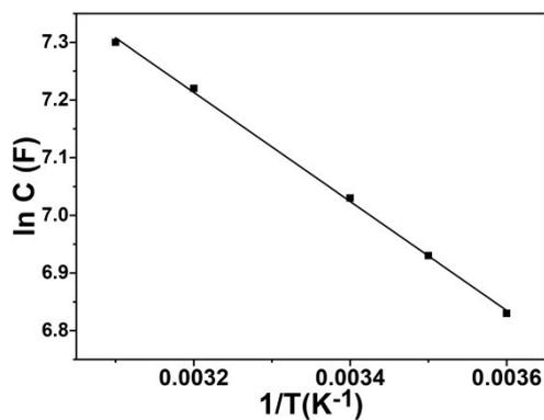
**Fig. S2** Electrochemical properties of PC-CDs-1.5% symmetrical capacitor in  $1\text{M H}_2\text{SO}_4/0.06\text{ M KI}$  electrolyte systems at different temperatures for Arrhenius linear relationship curve
