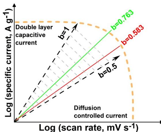
Fig. S6 The fitting plots between log (i) and log (v)
