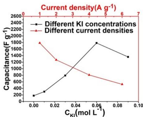
**Fig. S5** PC-CDs-1.5% based symmetric supercapacitor at different KI concentrations vs 0.06M KI at different current densities
