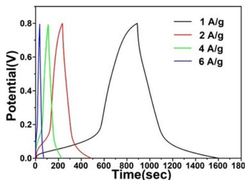
**Fig. S4** GCD curves of different current densities of PC-CDs-1.5% based symmetric supercapacitor in 1 M H<sub>2</sub>SO<sub>4</sub>/0.06 M KI electrolyte
