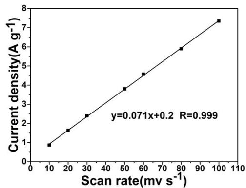
**Fig. S3** Electrochemical properties of PC-CDs-1.5% symmetrical capacitor in  $1\text{M H}_2\text{SO}_4$  electrolyte for current response curves at different voltage sweep speeds
