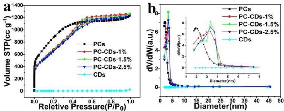
**Fig. S1** (a)  $\text{N}_2$  adsorption–desorption curves and (b) pore size distribution for the PC, CDs and PC-CDs-1, PC-CDs-1.5%, PC-CDs-2.5
