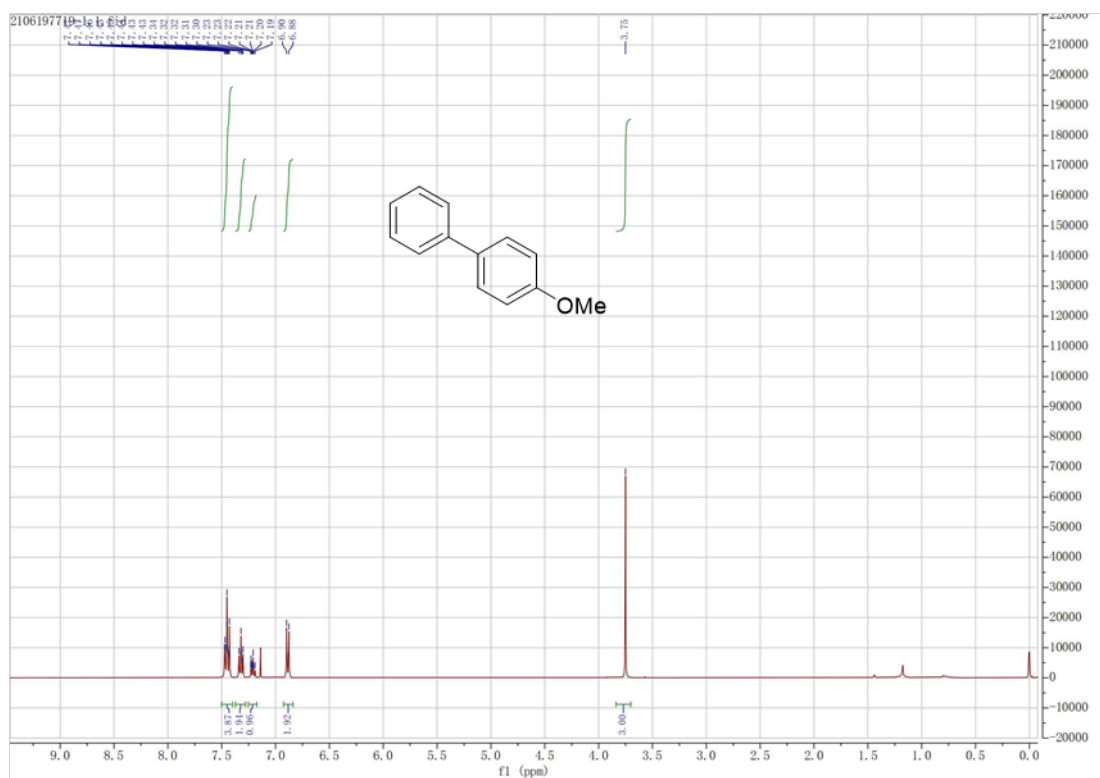
Figure S18. 1 H NMR of 4-methoxy-1,1'-biphenyl. 1 H NMR (600 MHz, CDCl 3 ) δ 7.43-7.47 (m, 4H), 7.30-7.34 (m, 2H), 7.19-7.23 (m, 1H), 6.88-6.89 (d, 2H), 3.75 (s, 3H).
