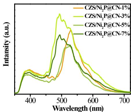
**Figure S4.** PL spectra of CZS/Ni<sub>2</sub>P@CN-*x* (*x* represents 1%, 3%, 5% and 7%)
