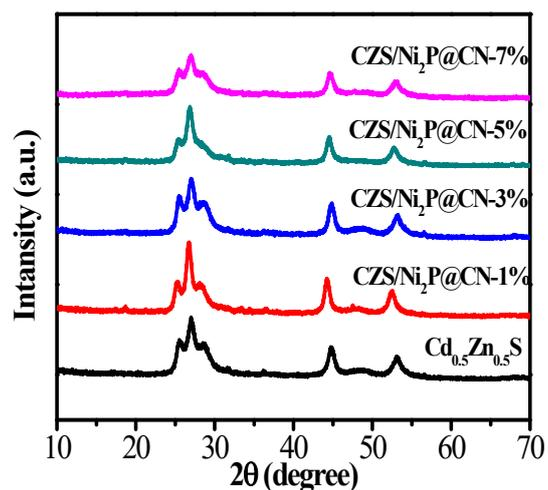
**Figure S2.** XRD patterns of CZS/Ni<sub>2</sub>P@CN-*x*% composites with various cocatalyst contents.
