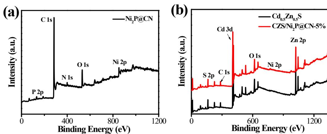
**Figure S3.** Survey XPS spectra of (a) Ni<sub>2</sub>P@CN, (b) CZS/Ni<sub>2</sub>P@CN-5% and Cd<sub>0.5</sub>Zn<sub>0.5</sub>S.
