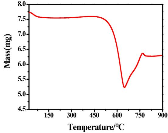
**Figure S1.** The TG curve of Ni<sub>2</sub>P@CN.
