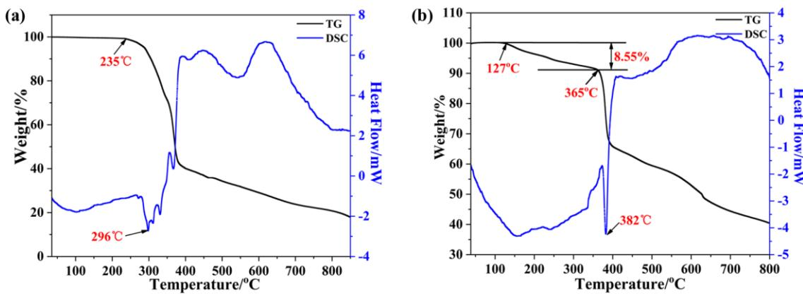
**Fig. S1** Thermo-gravimetric (TG) and Differential scanning calorimetry (DSC) curves of **1** and **2**.
