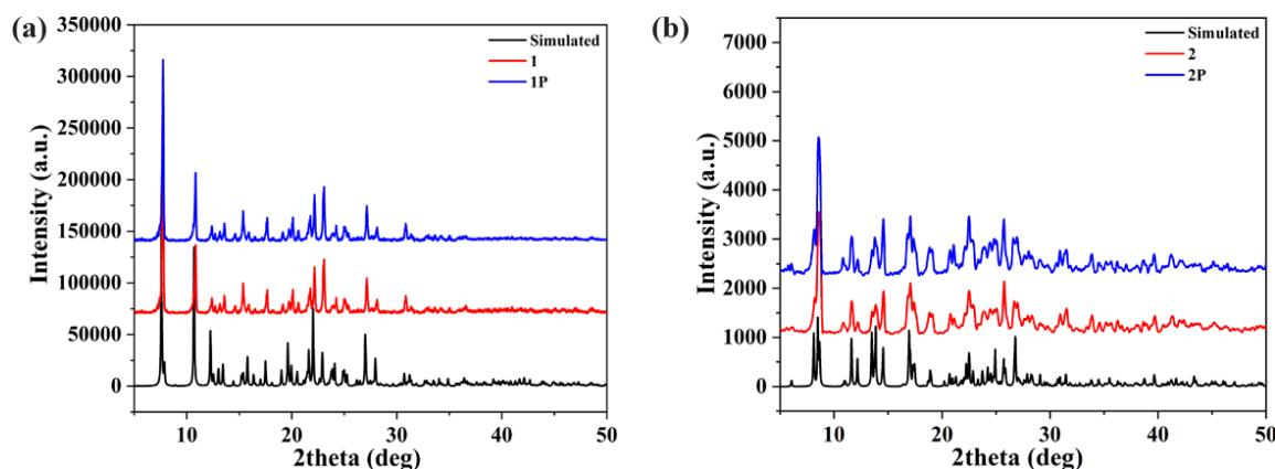
**Fig. S6** PXRD patterns of **1** and **2** simulated from the X-ray single-crystal structures, as-synthesized samples and after irradiation samples.
