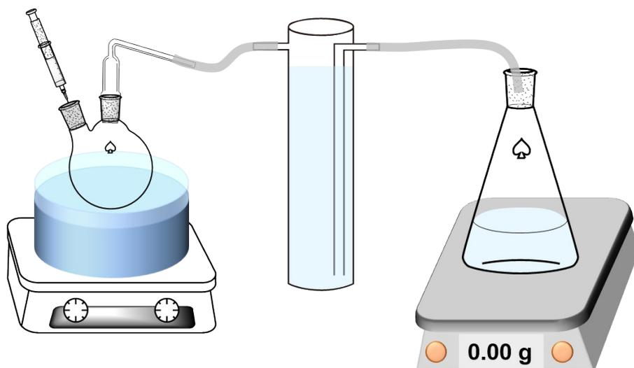
**Scheme S1.** Schematic of reaction system of H<sub>2</sub> generation from AB hydrolysis.
