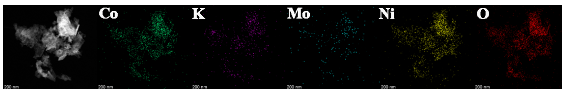
Fig. S7 EDX elemental mapping of Co, K, Mo, Ni, and O elements for act-NiMoO 4 -CoO/CC at -0.25 V.
