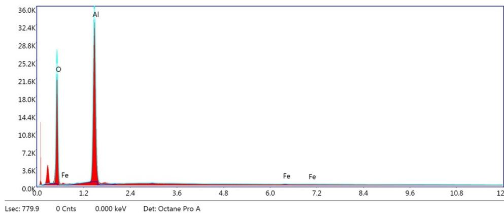
**Figure S3.** EDS spectrum of Fe/Al<sub>2</sub>O<sub>3</sub> platelets.
