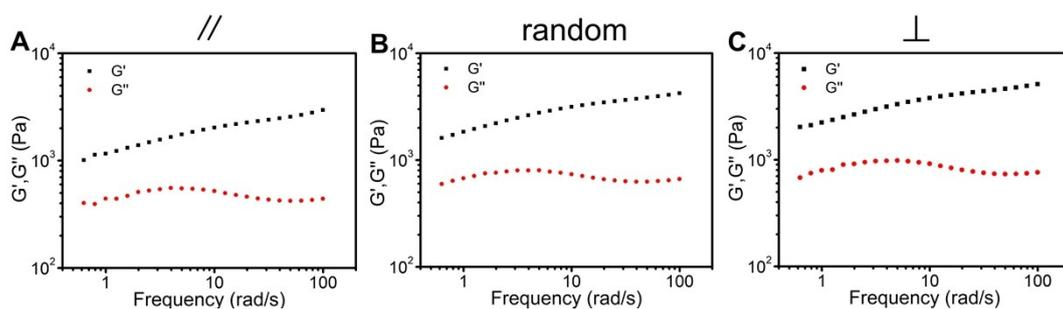
**Figure S6.** Frequency ( $\omega$ ) sweep tests at  $\omega = 0.1-100 \text{ rad s}^{-1}$  and strain ( $\gamma$ ) = 1.0% of Tb-containing hydrogel.
