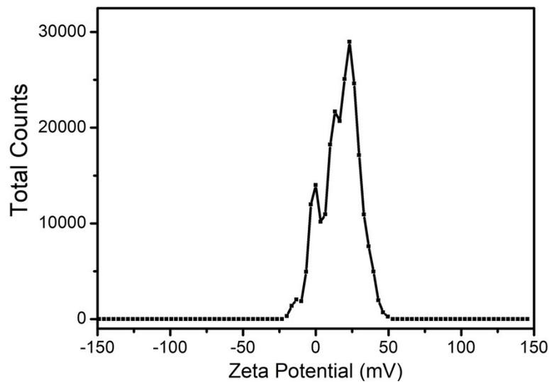
**Figure S2.** Zeta potential of pristine Al<sub>2</sub>O<sub>3</sub> platelets in deionized water ( $\zeta = 16.9$  mV).
