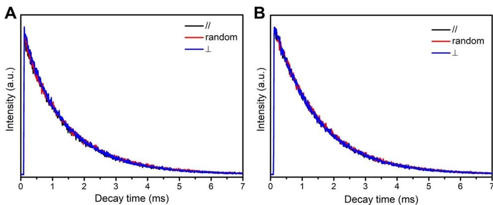
**Figure S10.** Decay curves of (A) Tb-containing (excited at 280 nm and monitored at 544 nm) and (B) Eu-containing (excited at 280 nm and monitored at 615 nm) hydrogel along different direction.
