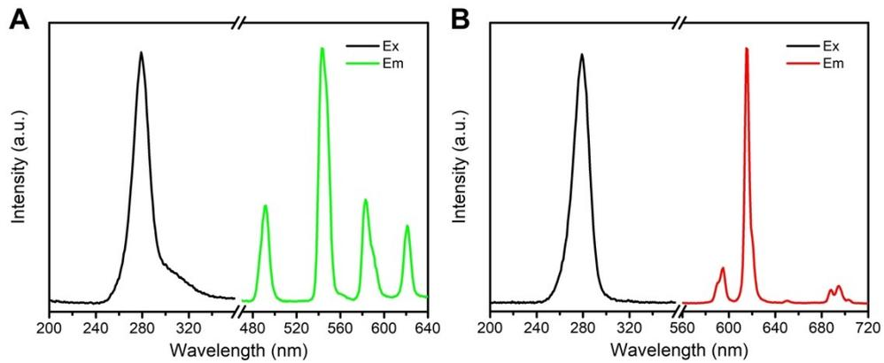
**Figure S9.** Normalized excitation ( $\lambda_{\text{mon}} = 544$  nm for Tb, 615 nm for Eu) (left) and emission ( $\lambda_{\text{ex}} = 280$  nm) (right) luminescence spectra of (A) Tb-containing and (B) Eu-containing hydrogel.
