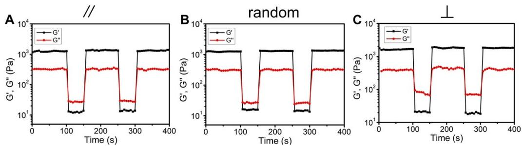
**Figure S8.** Continuous step strain test of Tb-containing hydrogel at  $\gamma = 0.1$  and 800% with  $\omega = 1.59$  Hz.
