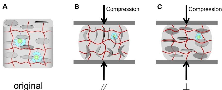
**Scheme S2.** Schematic illustration of Tb-containing hydrogel (A) original, compressive force was (B) parallel and (C) perpendicular to the oriented Fe/Al<sub>2</sub>O<sub>3</sub> platelets.
