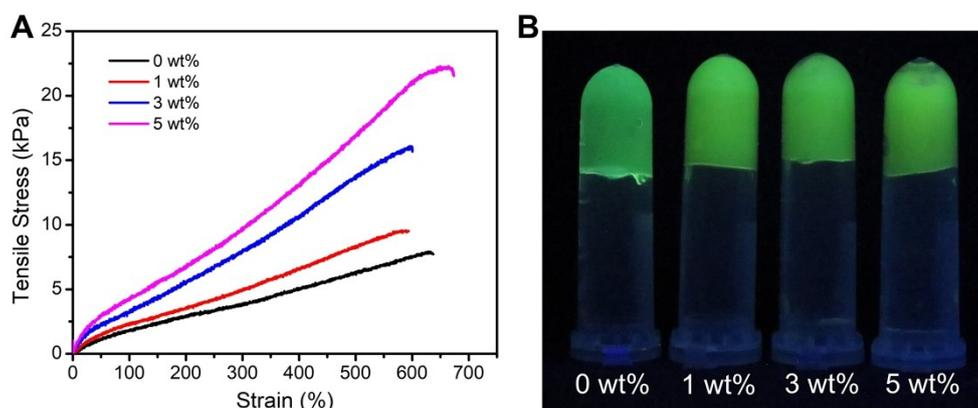
**Figure S5.** (A) Tensile stress-strain and (B) photos (under 254 nm UV light) of Tb-containing hydrogel with different contents of Fe/Al<sub>2</sub>O<sub>3</sub> platelets.
