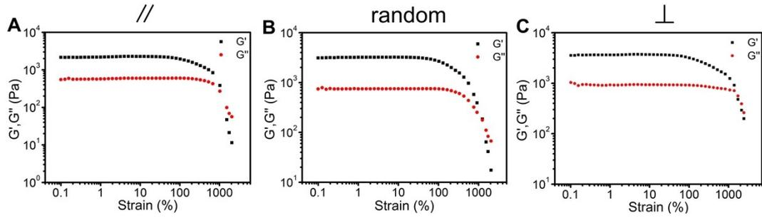
**Figure S7.** Strain sweep tests at  $\gamma = 0.1$ -2000% with  $\omega = 1.59$  Hz of Tb-containing hydrogel.
