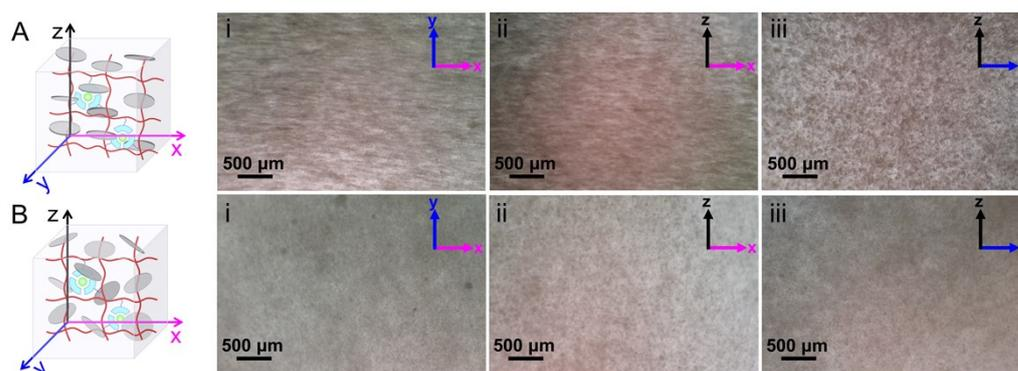
**Figure S4.** Optical microscope images of Tb-containing hydrogel in different directions.
