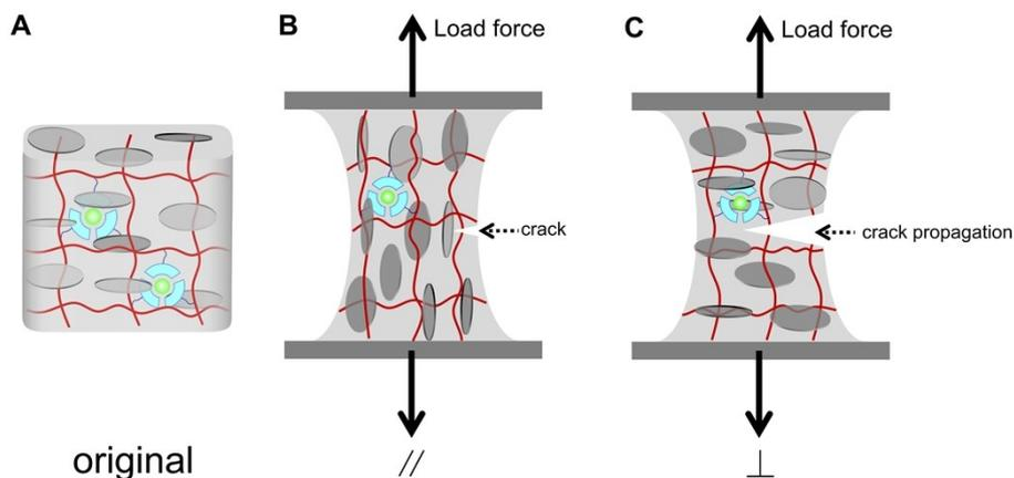
**Scheme S1.** Schematic illustration of Tb-containing hydrogel (A) original, tensile force was (B) parallel and (C) perpendicular to the oriented Fe/Al<sub>2</sub>O<sub>3</sub> platelets.
