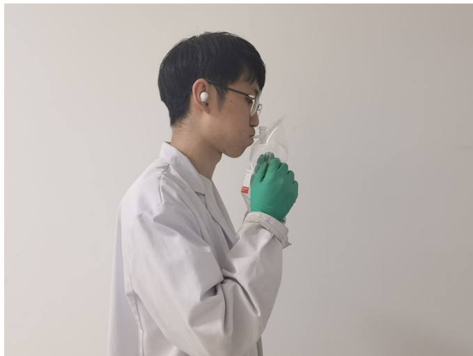
Fig. S3. Exhaled breath collected from a subject using a fluorine membrane collection bag.
