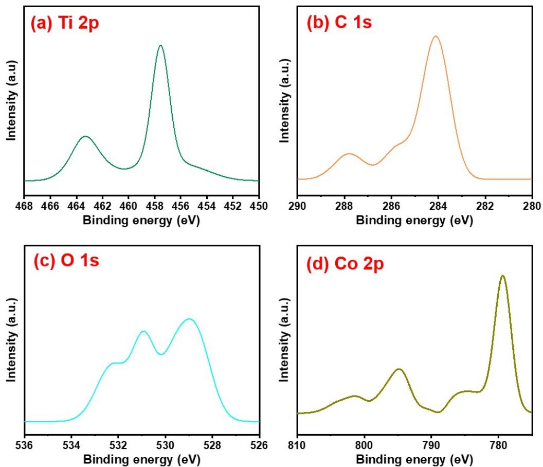
**Figure S10.** XPS profiles after 24 h overall water splitting for MXene/Co<sub>3</sub>O<sub>4</sub> composites: (a) Ti 2p, (b) C 1s, (c) O 1s and (d) Co 2p regions
