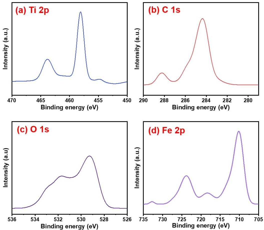
**Figure S11.** XPS profiles after 24 h overall water splitting for MXene/Fe<sub>3</sub>O<sub>4</sub> composites: (a) Ti 2p, (b) C 1s, (c) O 1s and (d) Fe 2p regions
