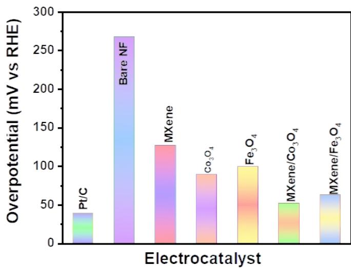
**Figure S6.** HER overpotential for bare NF, Pt/C, MXene, Co<sub>3</sub>O<sub>4</sub>, Fe<sub>3</sub>O<sub>4</sub>, MXene/Co<sub>3</sub>O<sub>4</sub>, and MXene/Fe<sub>3</sub>O<sub>4</sub> composites
