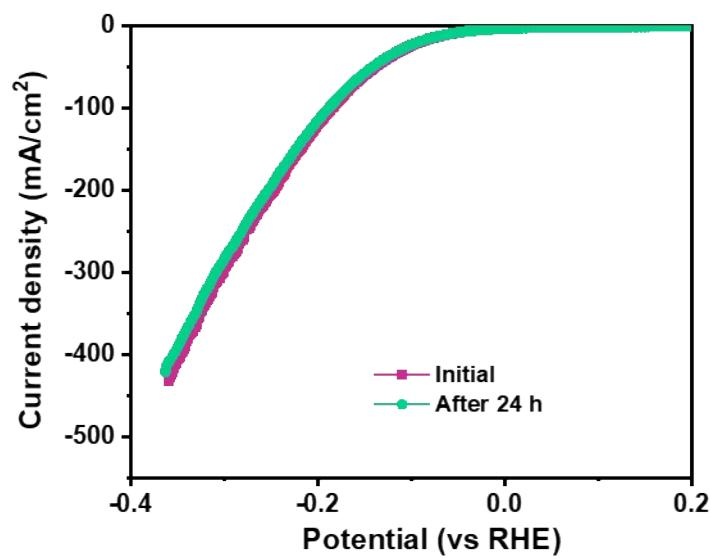
**Figure S7.** LSV profiles before and after 24 h continuous OER reaction
