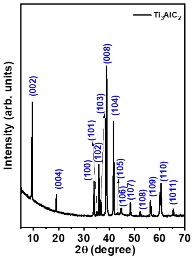
**Figure S1.** XRD pattern of MAX phase  $\text{Ti}_3\text{AlC}_2$ .
