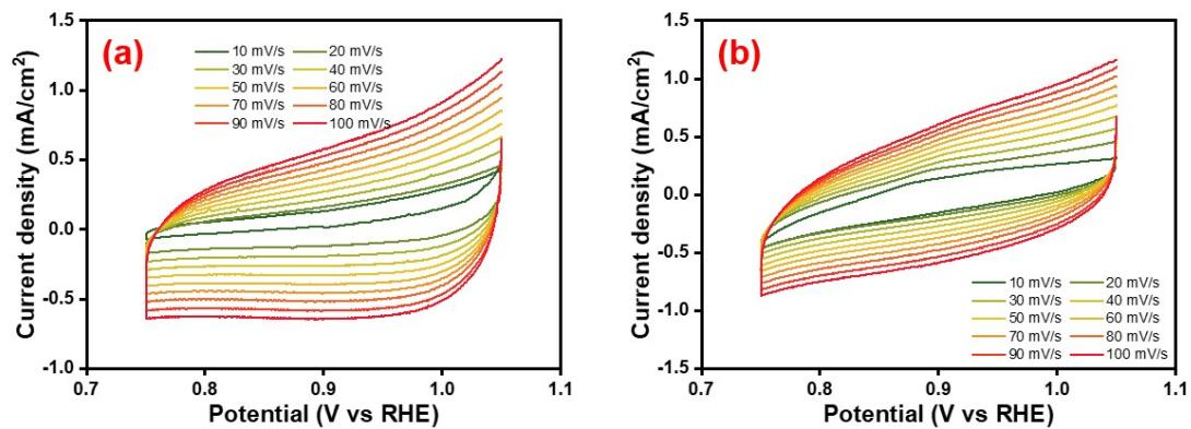
**Figure S9.** Non-faradaic region CVs for the(a) MXene/Co<sub>3</sub>O<sub>4</sub> and (b) MXene/Fe<sub>3</sub>O<sub>4</sub> nanocomposites at different scan rates.
