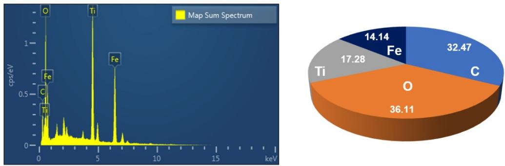
**Figure S5.** EDX spectrum and their composition chart for MXene/Fe<sub>3</sub>O<sub>4</sub> nanocomposites
