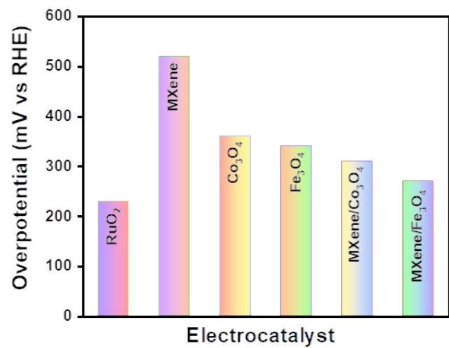
**Figure S8.** OER overpotential for RuO<sub>2</sub>, MXene, Co<sub>3</sub>O<sub>4</sub>, Fe<sub>3</sub>O<sub>4</sub>, MXene/Co<sub>3</sub>O<sub>4</sub>, and MXene/Fe<sub>3</sub>O<sub>4</sub> composites
