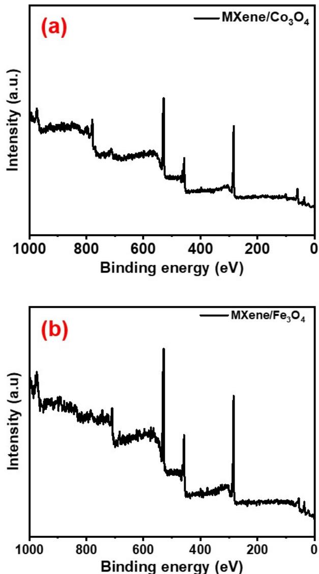
**Figure S3.** XPS survey spectra for the (a) MXene/Co<sub>3</sub>O<sub>4</sub> and (b) MXene/Fe<sub>3</sub>O<sub>4</sub> nanocomposites.
