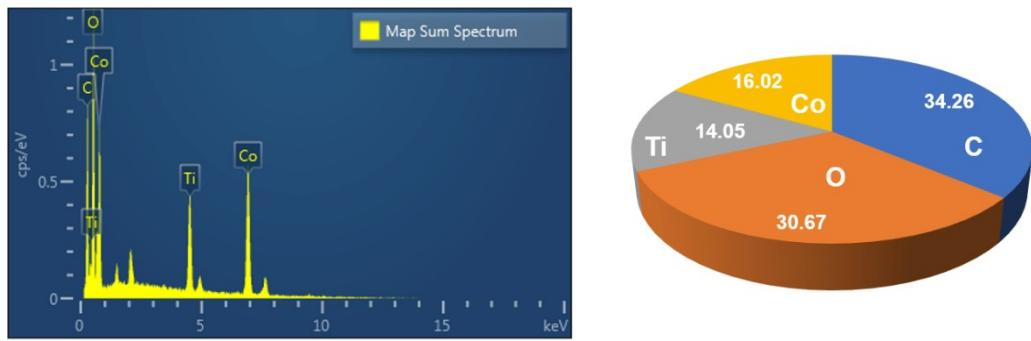
**Figure S4.** EDX spectrum and their composition chart for MXene/Co<sub>3</sub>O<sub>4</sub> nanocomposites
