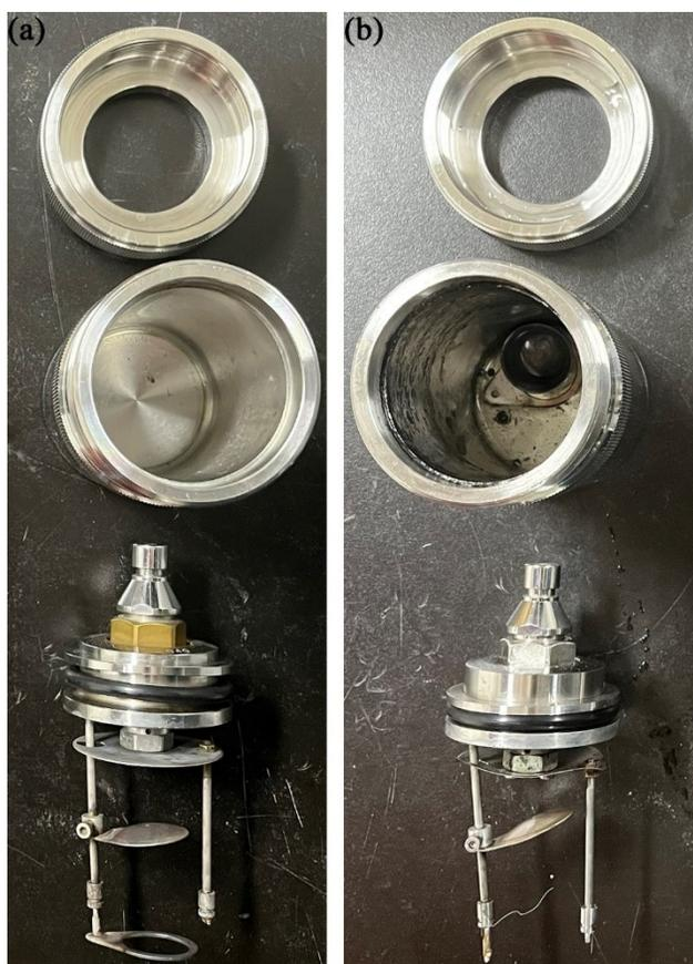
**Fig. S6** (a) The complete oxygen bomb. (b) The Oxygen bomb destroyed by explosion.
