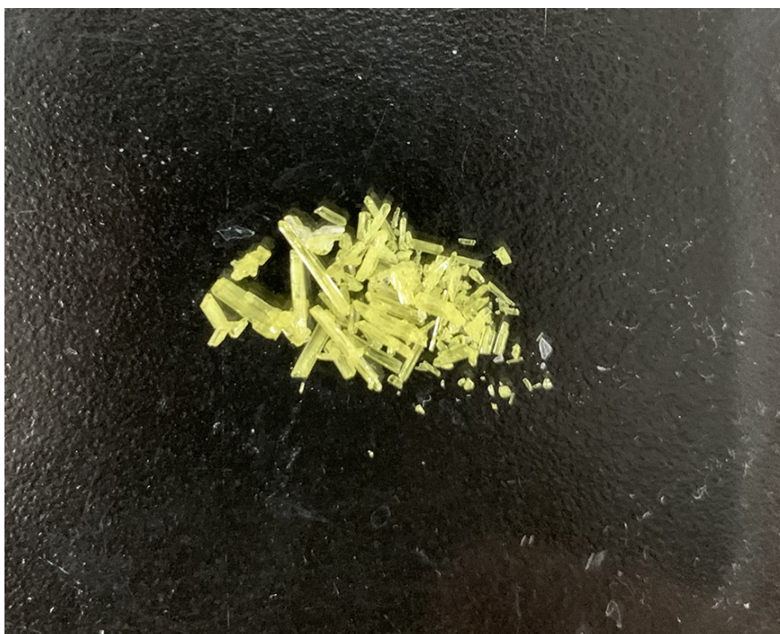
Figure S4. Photograph of crystals grown in a solution with M_{\text{Sb}^{3+}}/M_{(\text{Bi}^{3+}+\text{Sb}^{3+})} of 40%.
