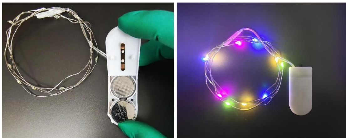
Figure S24 Digital photos of a light-emitting diode (LED) four-color lamp string lit up by CR2025-type lithium-sulfur batteries with \text{CoS}_2/\text{NC}@1\text{T MoS}_2\text{-PP} separator.
