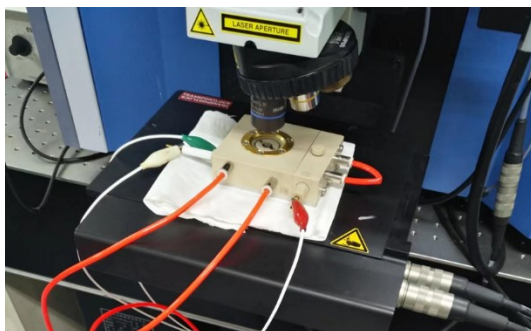
Fig. S15. The experimental set up for the in situ Raman spectroscopy measurement.
