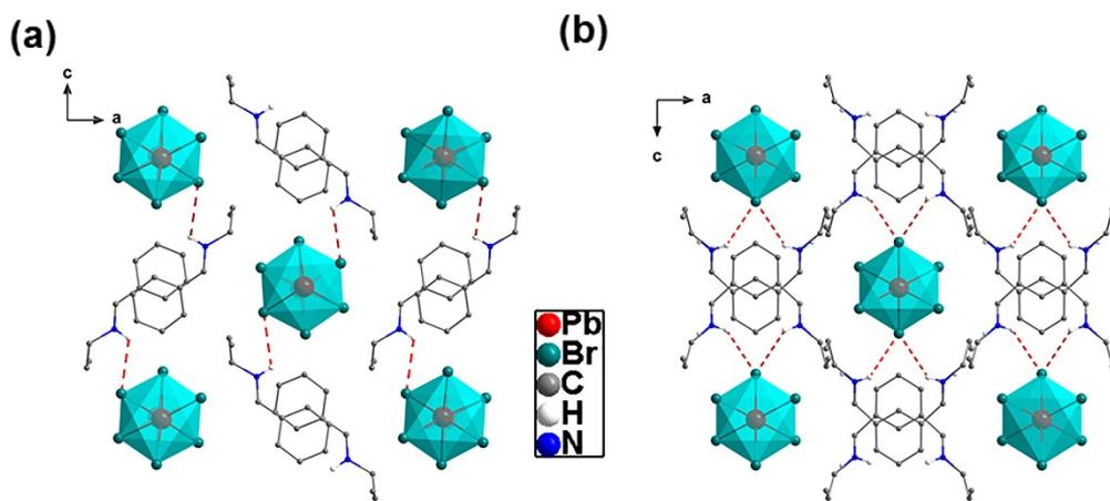
**Figure S7.** The N- H...Br hydrogen-bonding interactions between organic cations and inorganic framework in compound **1** were showed at a) LTP and b) HTP. Some hydrogen bonds were omitted for clarity.
