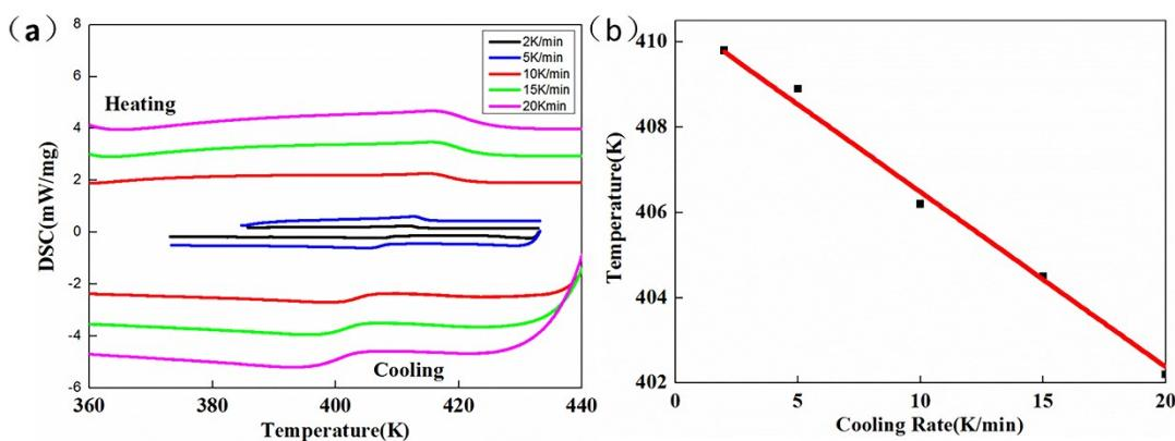
**Figure S6.** a) Differential scanning calorimetry of **1** at different heating/cooling rate. b) The actual phase transition point confirmed by extrapolating intercept of the plot of peak points at different heating/cooling rates and is finally measured to be 411 K.
