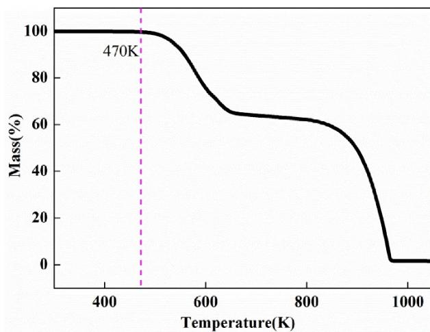
**Figure S5.** The TG curves of 1. This compound can maintain the thermal stable up to 470 K.
