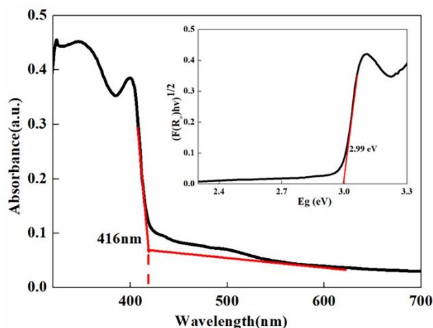
**Figure S8.** The UV/vis absorption spectrum of **1**, the absorption edge of this compound is estimated to be 420 nm.
