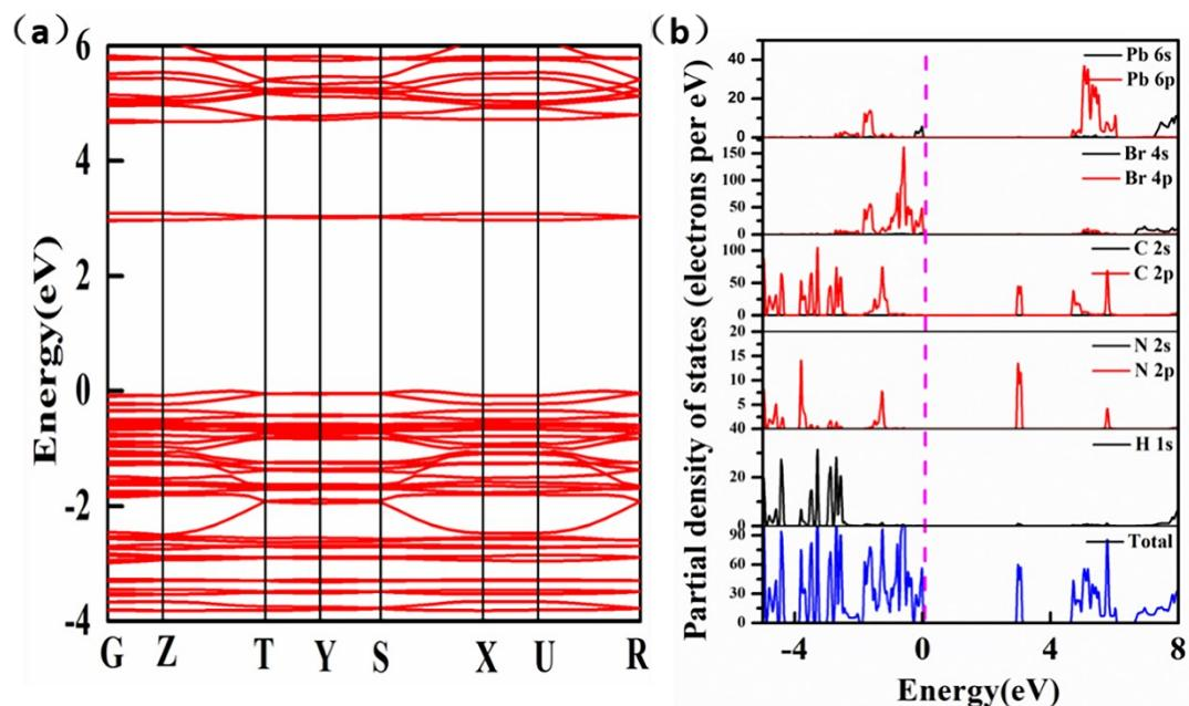
**Figure S10.** a) Electronic band structure and b) partial density of states for **1**.
