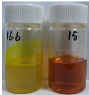
Figure S32. Photos of supernatant of Entry 15 and 16. The deionized water was firstly added to the reaction mixture and then extracted with diethyl ether to get the supernatant.
