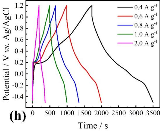
**Fig. S3.** CV curves at varied scan rates and GCD curves at 0.4-2.0 A g<sup>-1</sup> of (a, b) MnO<sub>2</sub>, (c, d) Co-MnO<sub>2</sub>-1, (e, f) Co-MnO<sub>2</sub>-3, and (g, h) Co-MnO<sub>2</sub>-4.
