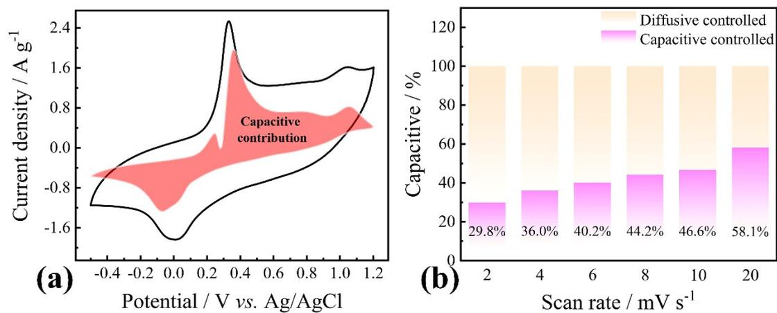
**Fig. S4.** (a) CV curve with the capacitive contribution at a scan rate of 10 mV s<sup>-1</sup>, (b) the percentages of capacitive and diffusion contributions of MnO<sub>2</sub>.
