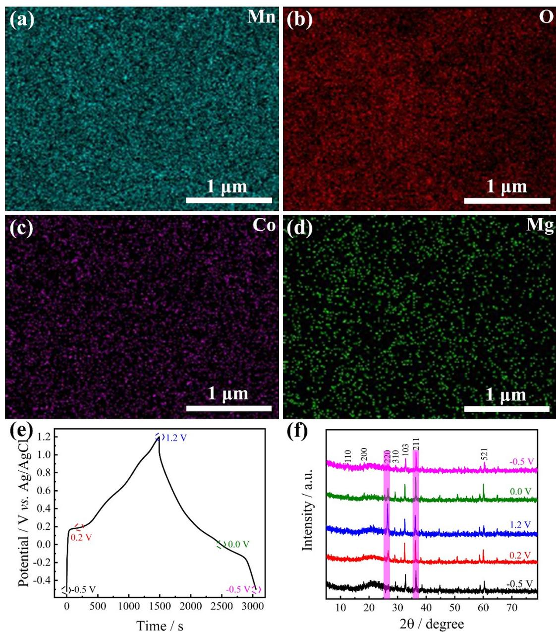
**Fig. S6.** Elemental mapping images of (a) Mn, (b) O, (c) Co, and (d) Mg of Co-MnO<sub>2</sub>-2 electrode charged to 1.2 V. (e) GCD curve of Co-MnO<sub>2</sub>-2 at 0.5 A g<sup>-1</sup>, (f) XRD pattern of Co-MnO<sub>2</sub>-2 electrode during the charge/discharge process.
