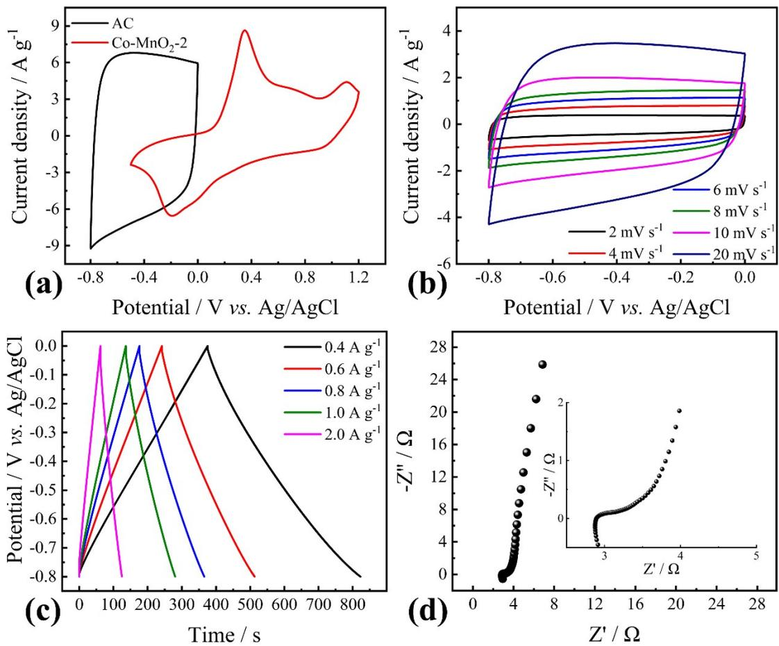
**Fig. S7.** (a) CV curves of AC and Co-MnO<sub>2</sub>-2 at a scan rate of 10 mV s<sup>-1</sup>. (b) CV curves at 2-20 mV s<sup>-1</sup>, (c) GCD curve at 0.5-2.0 A g<sup>-1</sup>, and (d) Nyquist plot of AC.
