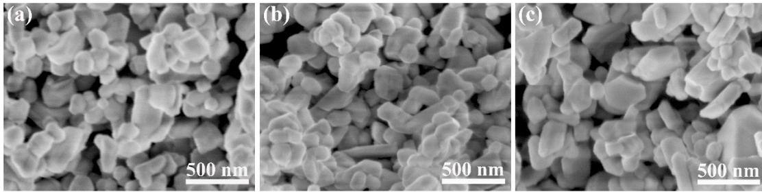
**Fig. S1.** SEM images of (a) Co-MnO<sub>2</sub>-1, (b) Co-MnO<sub>2</sub>-3, and (c) Co-MnO<sub>2</sub>-4.
