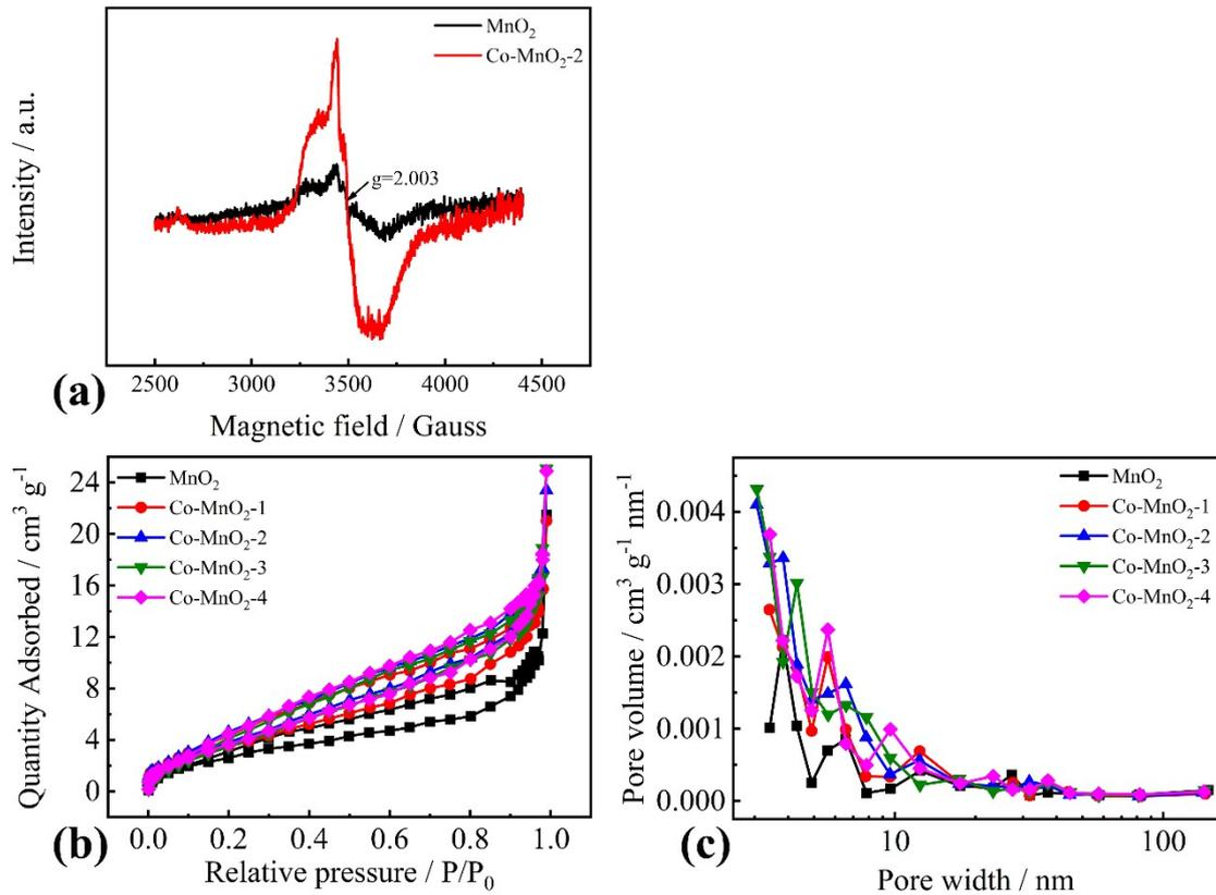
**Fig. S2.** (a) EPR spectra for the MnO<sub>2</sub> and Co-MnO<sub>2</sub>-2. (b) BET adsorption-desorption isotherms and (c) pore size distributions of MnO<sub>2</sub>, Co-MnO<sub>2</sub>-1, Co-MnO<sub>2</sub>-2, Co-MnO<sub>2</sub>-3, and Co-MnO<sub>2</sub>-4.
