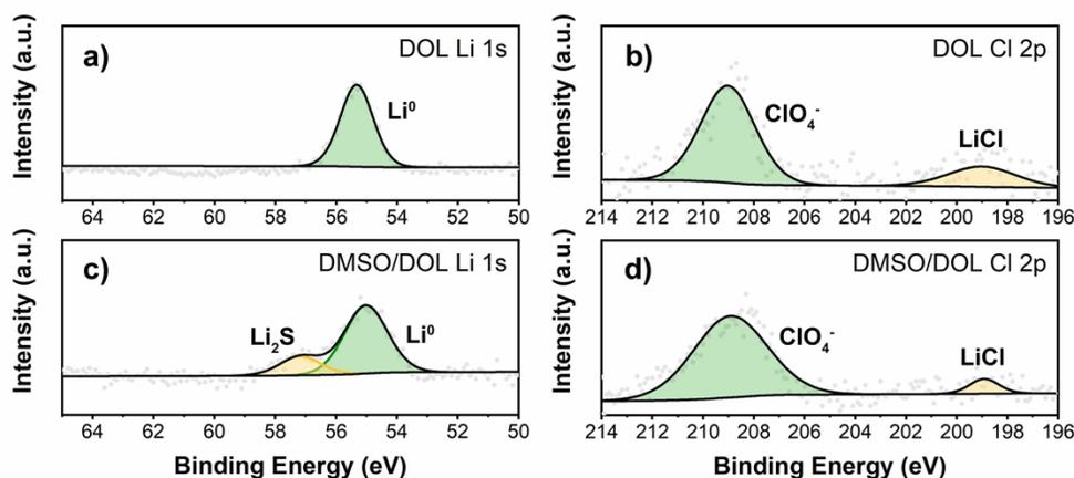
**Figure S8.** High resolution Li 1s and Cl 2p XPS spectra for the SEI formed on Li metal anode in Li/Li symmetric cells after 5 cycles at  $0.5 \text{ mA cm}^{-2}$  and  $1 \text{ mA h cm}^{-2}$  at RT with DOL electrolyte and DMSO/DOL electrolyte, respectively.
