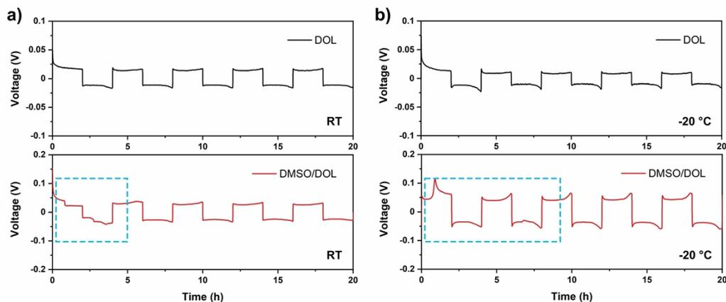
**Figure S6.** The first 20 hours of cycling in Li/Li symmetric cells with DOL electrolyte and DMSO/DOL electrolyte at a) RT; b) -20 °C, at 0.5 mA cm<sup>-2</sup>, 1mA h cm<sup>-2</sup>. The fluctuation labelled by the blue box represents the stabilization process in DMSO added electrolytes.
