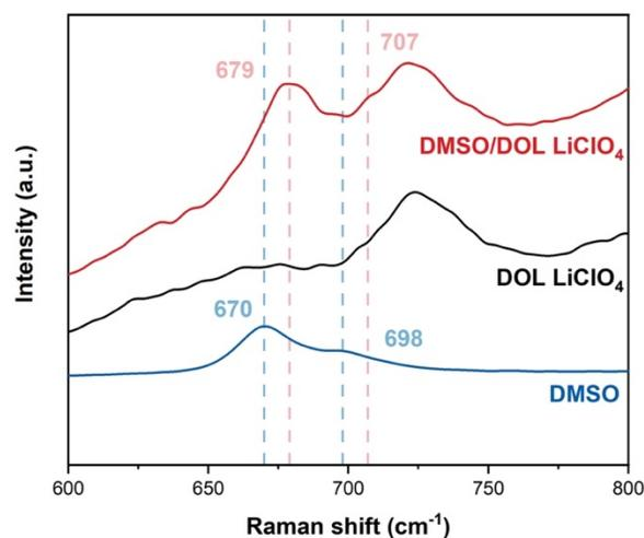
**Figure S5.** Raman spectroscopy of pure DMSO, DOL/LiClO<sub>4</sub> electrolyte, and DOL/LiClO<sub>4</sub> electrolyte with 5 vol% DMSO. The blue dotted lines represent two characteristic peaks of DMSO, while the red dotted lines labelled the shifted peaks in the DMSO added DOL/LiClO<sub>4</sub> electrolyte.
