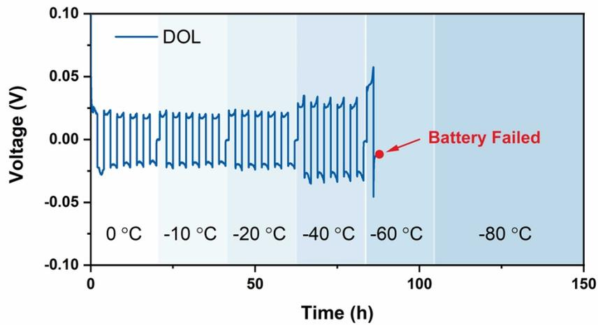
**Figure S2.** Step-wise cycling tests in Li/Li symmetric cells with DOL electrolyte under varying temperatures from  $0 \text{ }^{\circ}\text{C}$  to  $-80 \text{ }^{\circ}\text{C}$  at  $0.25 \text{ mA cm}^{-2}$  and  $0.5 \text{ mA h cm}^{-2}$ . The cell failed at  $-60 \text{ }^{\circ}\text{C}$ .
