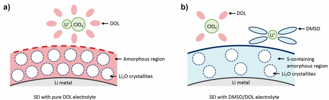
**Figure S9.** Proposed schemes of the solvation behavior of Li ion and the structure of the SEI in a) pure DOL electrolyte and b) DMSO/DOL electrolyte, respectively.
