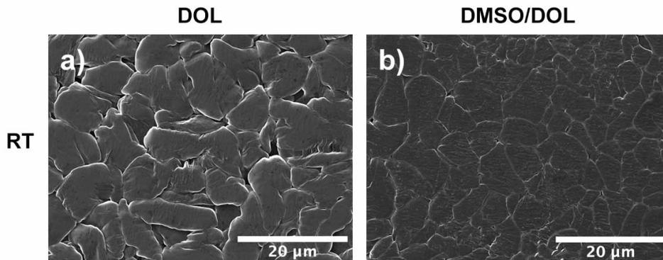
**Figure S3.** The morphology of deposited Li metal on Cu substrate at  $0.5 \text{ mA cm}^{-2}$  for 8 hours at RT with a) DOL electrolyte and b) DMSO/DOL electrolyte.
