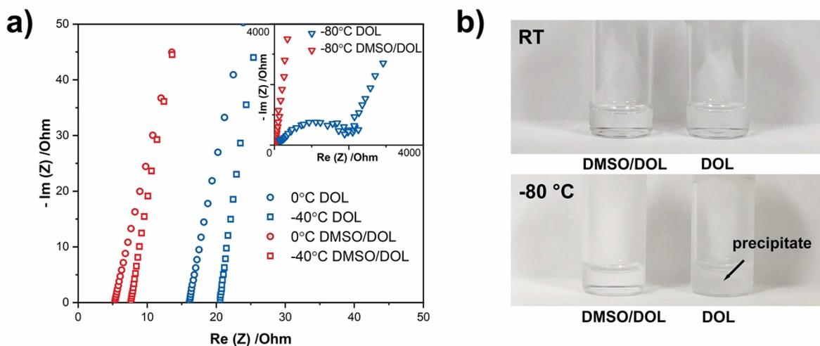
**Figure S4.** a) EIS plots of DOL and DMSO/DOL electrolytes in SS/SS cells, respectively, at different temperatures at 0 °C, -40 °C, and -80 °C (inset). b) The digital photos of DOL and DMSO/DOL electrolytes after stored at RT and -80 °C overnight. Li salt precipitated in DOL electrolyte at -80 °C.
