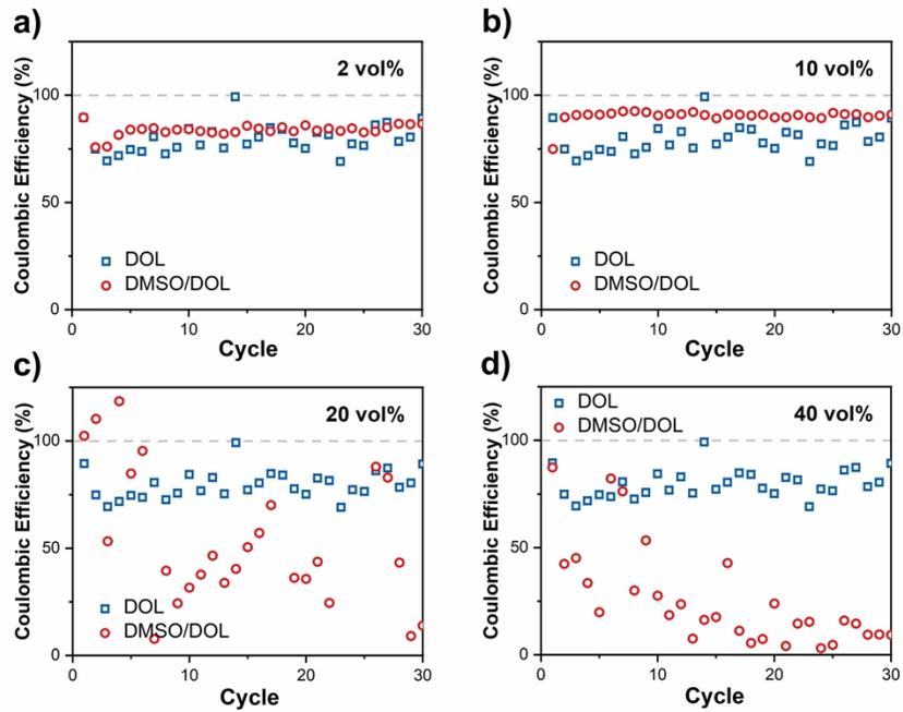
**Figure S1.** The CE of DMSO/DOL electrolyte at RT with a) 2 vol%; b) 10 vol%; c) 20 vol%; and d) 40 vol% of DMSO at  $0.5 \text{ mA cm}^{-2}$  and  $1 \text{ mA h cm}^{-2}$ .
