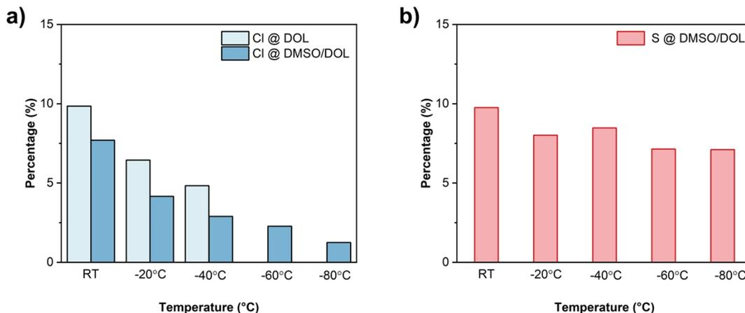
**Figure S7.** EDX results of the SEI formed on Li metal anode after 5 cycles of Li plating and stripping in Li/Li cells at  $0.5 \text{ mA cm}^{-2}$  and  $1 \text{ mA h cm}^{-2}$ . a) The percentage of the Cl in the SEI formed in DOL electrolyte from RT to  $-40 \text{ }^\circ\text{C}$  and in DMSO/DOL electrolyte from RT to  $-80 \text{ }^\circ\text{C}$ . b) The percentage of S in SEI formed in DMSO/DOL electrolyte from RT to  $-80 \text{ }^\circ\text{C}$ .
