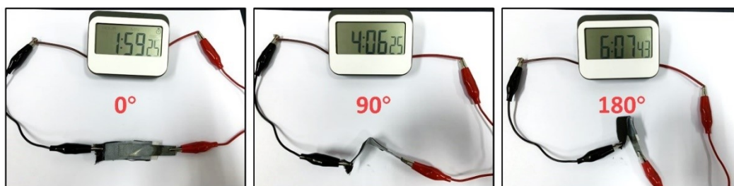
Fig. S27. Photographs of a timer powered by one flexible solid-state ZAB based on Fe-SA/BNC under different bending degrees.
