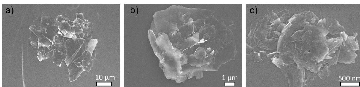
Figure S1. Ball-milled graphite samples. a) EG4, b) GFMN10.54 and c) GFMN126.
