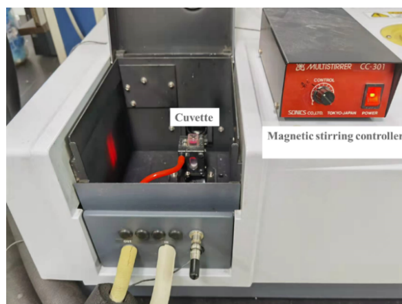
Figure S11. Photograph of a set-up used to record the fluorescence spectra of NR-borne MCM-41 particles under magnetic stirring.
