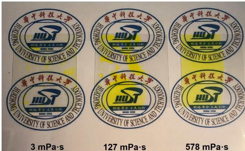
**Figure S16.** Effect of viscosity on the coating properties on PET films.
