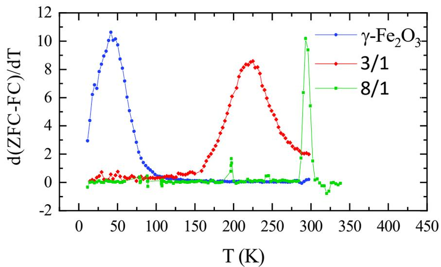
**Figure S8.** Derivative of ZFC measurements with temperature to obtain the average  $T_B$  for  $\gamma\text{-Fe}_2\text{O}_3$  seeds and  $\gamma\text{-Fe}_2\text{O}_3$ @CoO NP with molar ratios OAc/Co = 3/1 and 8/1.
