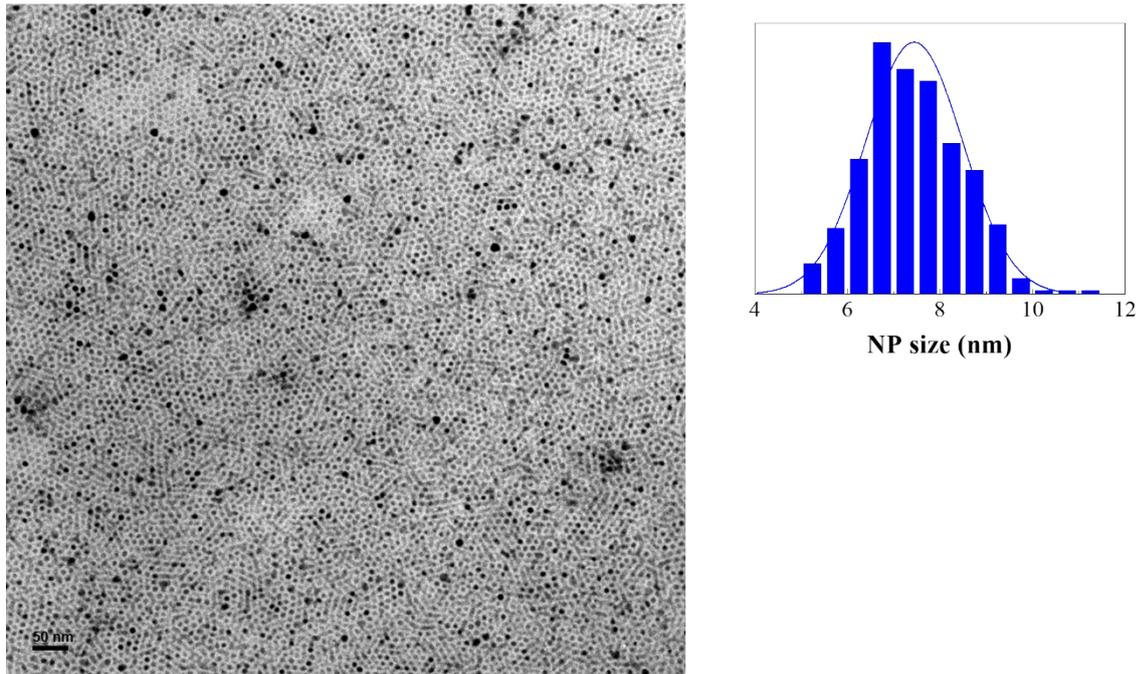
**Figure S7.** TEM micrograph and size distribution of cobalt oxide nanoparticles grown without the presence of iron oxide seeds with a molar ratio OAc/Co = 3/1.
