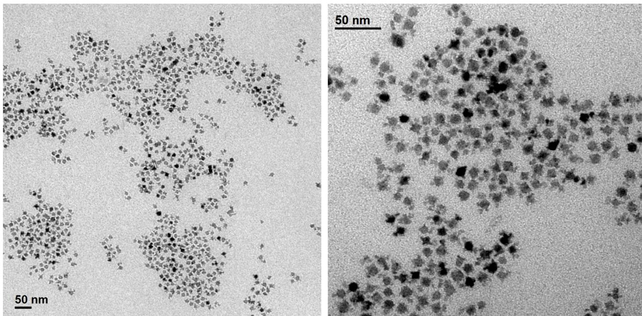
**Figure S3.** TEM micrographs of  $\gamma\text{-Fe}_2\text{O}_3\text{@CoO}$  NPs synthesized with a molar ratio  $\text{OAc/Co} = 2/1$ .
