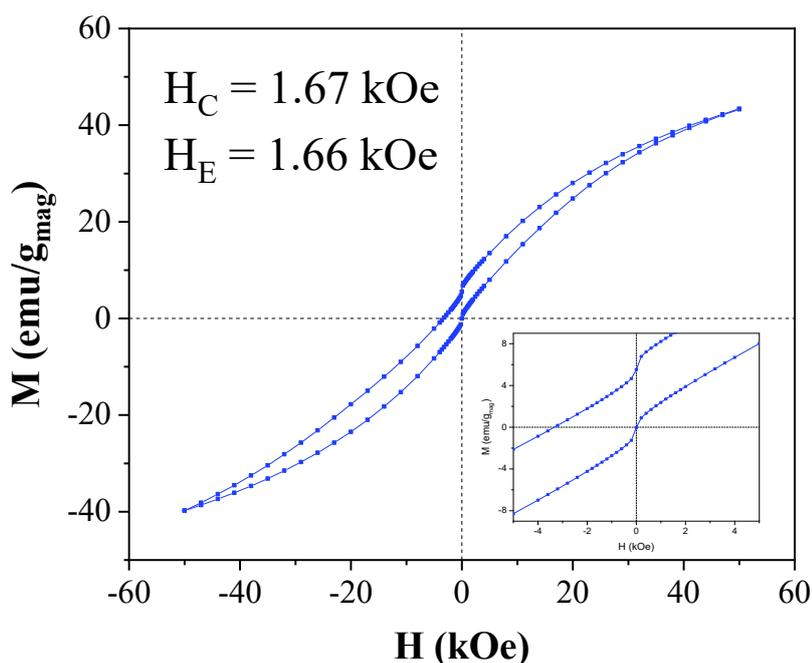
**Figure S9.** Hysteresis loop measured at 5 K after field-cooling (50 kOe) for  $\gamma$ -Fe<sub>2</sub>O<sub>3</sub> @CoO NP with molar ratio OAc/Co = 3/1. Inset: Detail of the hysteresis loop when crossing the axes.
