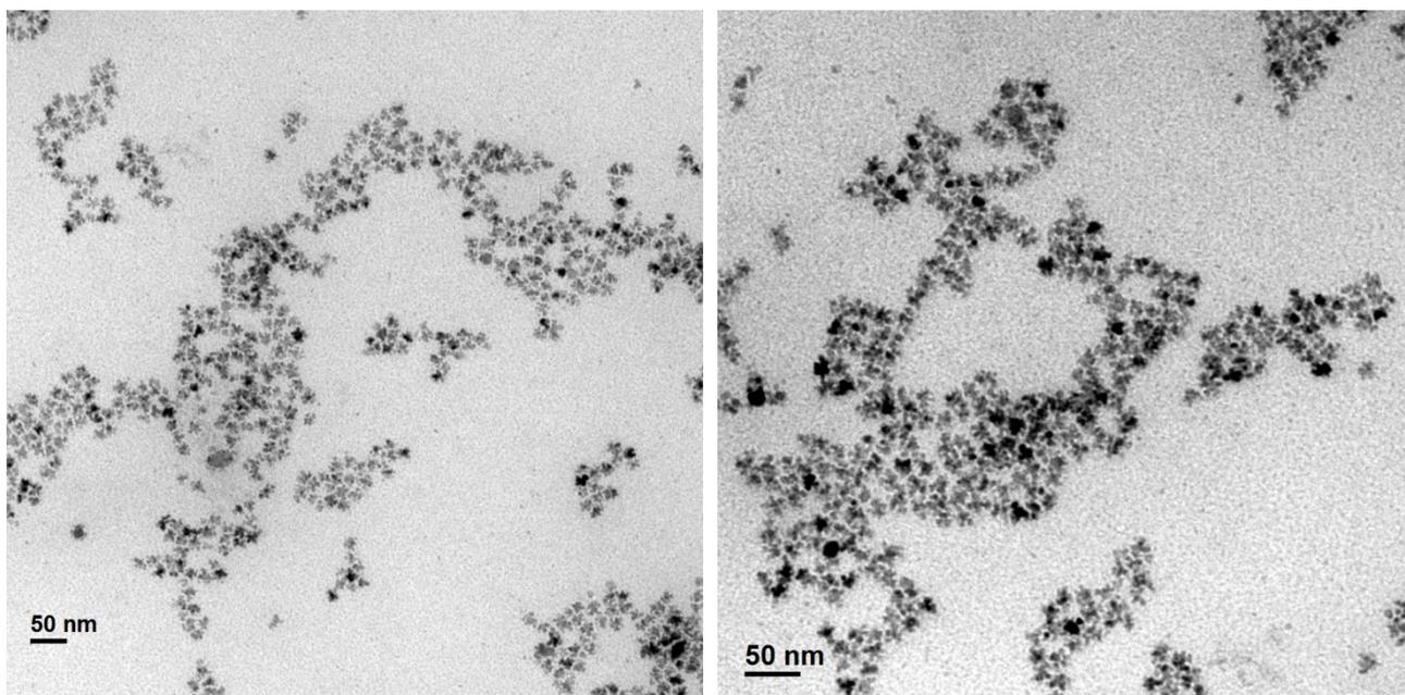
**Figure S6.** TEM micrographs of  $\gamma\text{-Fe}_2\text{O}_3@CoO$  NPs synthesized with a molar ratio OAc/Co = 8/1.
