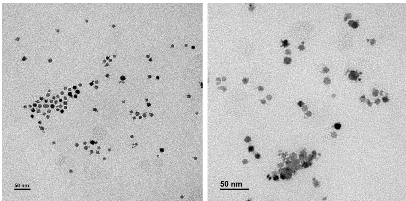
**Figure S2.** TEM micrographs of  $\gamma\text{-Fe}_2\text{O}_3\text{@CoO}$  NPs synthesized with a molar ratio OAc/Co = 1/1.
