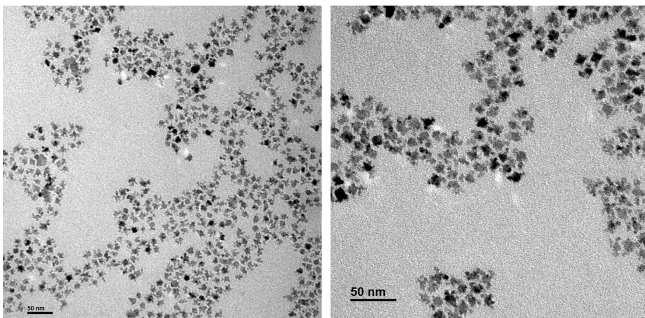
**Figure S4.** TEM micrographs of  $\gamma\text{-Fe}_2\text{O}_3\text{@CoO}$  NPs synthesized with a molar ratio  $\text{OAc/Co} = 3/1$ .
