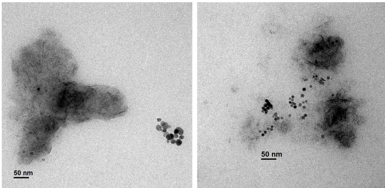
**Figure S1.** TEM micrographs of  $\gamma\text{-Fe}_2\text{O}_3\text{@CoO}$  NPs synthesized with a molar ratio OAc/Co = 0/1.
