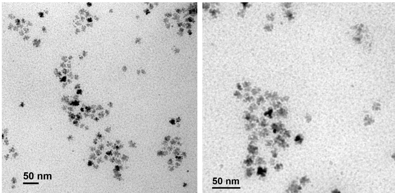
**Figure S5.** TEM micrographs of  $\gamma\text{-Fe}_2\text{O}_3@CoO$  NPs synthesized with a molar ratio OAc/Co = 5/1.
