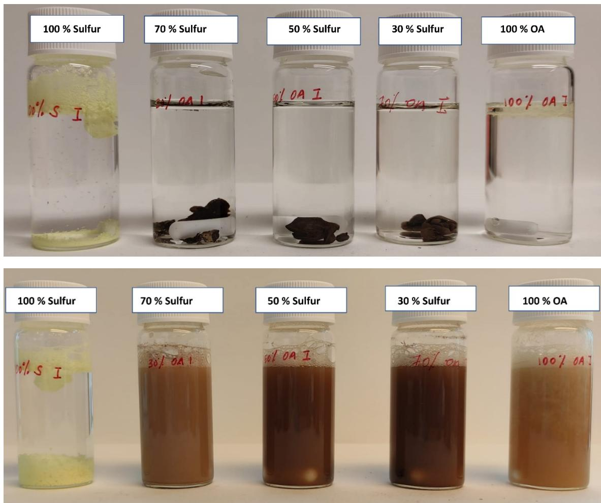
Figure S4: Photograph of batch experiment on selectivity studies before and after adsorption are shown above and below respectively. 25 mg L<sup>-1</sup> 20 mL aqueous mixed metal solutions treated with 100 % sulfur, Poly(S-70 %-OA), Poly(S-50 %-OA), Poly(S-30 %-OA), 100 % oleylamine are shown from left to right.
