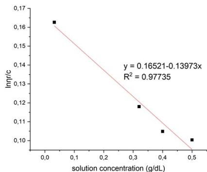
Figure S7: Intrinsic viscosity plot of the 50:50 sulfur:oleylamine polymer using THF as the solvent.
