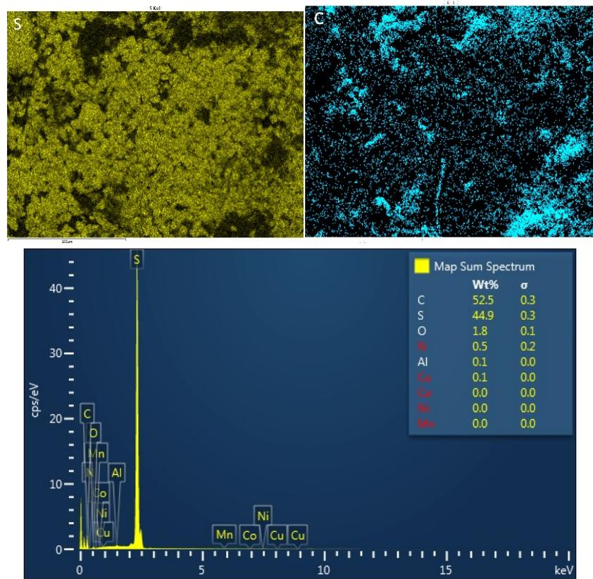
Figure S6: SEM-EDX mapping of the sulfur-oleylamine copolymer adsorbent after adsorption.
