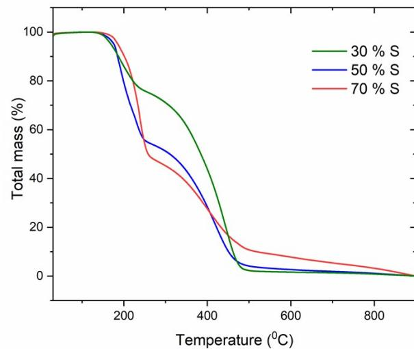
Figure S3: Thermogravimetric analysis (TGA) of sulfur-oleylamine copolymer with varied sulfur content (wt %). Green, blue and red line denotes Poly(S-30 %-OA), Poly(S-50 %-OA) and Poly(S-70 %-OA) respectively.
