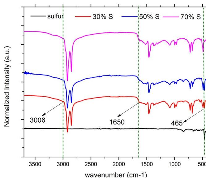
Figure S2: AT-FTIR spectra of sulfur-oleylamine copolymer with varied sulfur content (wt %) in comparison with sulfur. Green, blue, red and black line denotes Poly(S-30 %-OA), Poly(S-50 %-OA), Poly(S-70 %-OA), and elemental sulfur respectively.
