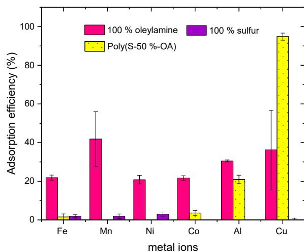
Figure S5: Metal selectivity profile in terms of adsorption efficiency (%). 100 % sulfur and 100 % oleylamine are monomers, done as control experiments.
