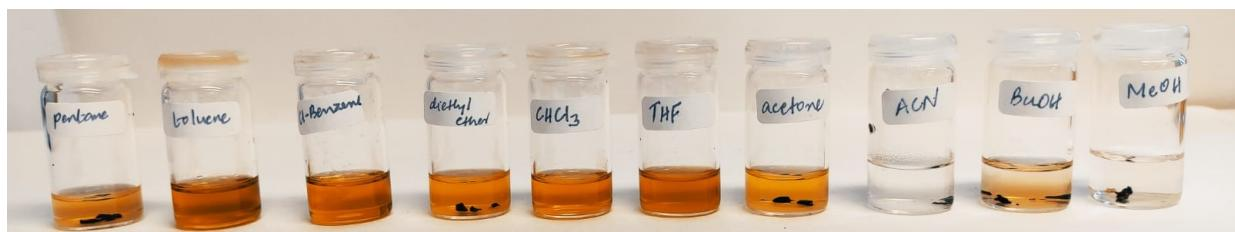
Figure S1: Solubility of Poly(S-50 %-OA) with increasing solvent polarity 10 mg in 2 mL solvent. From left to right the solvents are pentane, toluene, chloro-benzene, diethyl ether, chloroform, tetrahydrofuran, acetone, acetonitrile, butanol and methanol.
