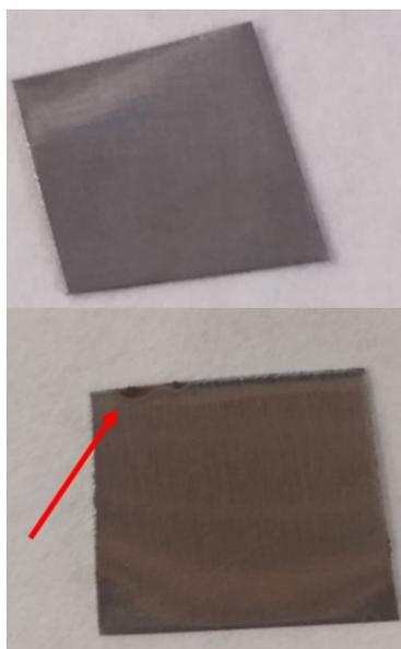
Figure S4: a109 low-carbon steel before (top) and after (bottom) five days of exposure to DMF-based corrosive solution containing 10%v H<sub>2</sub>O. Though effects of corrosion are visible, no significant change in fluorescence emission intensity was detected in the solution. The squares are 400 mg mass before corrosion and roughly 2 x 2 cm in size.
