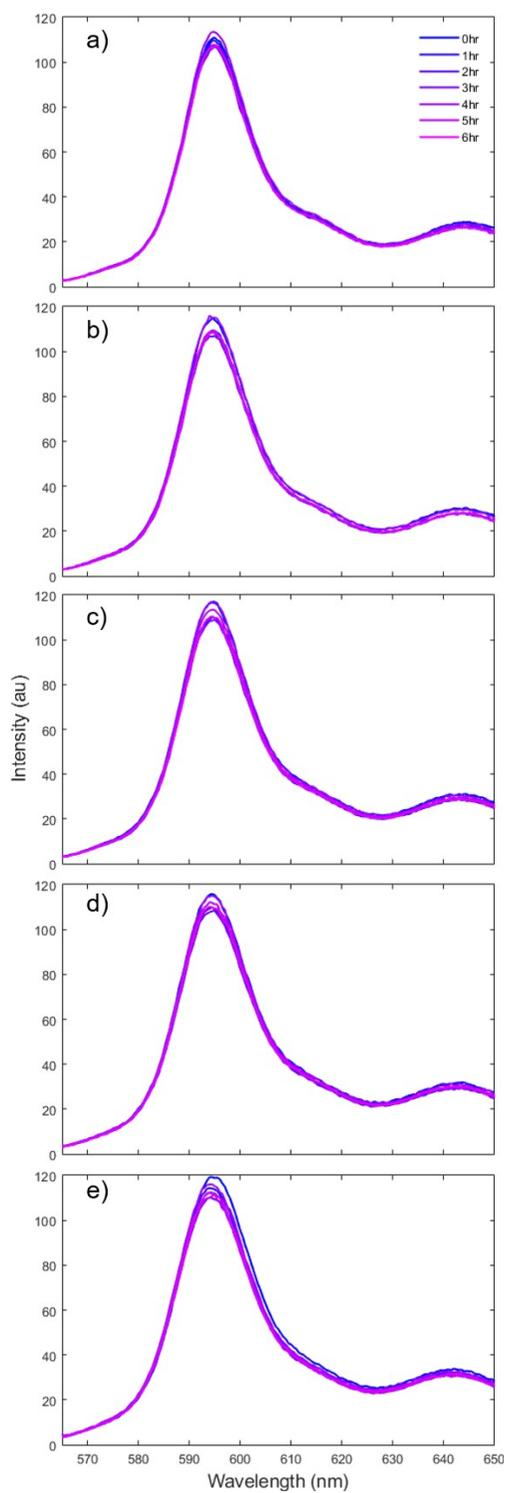
Figure S10: Fluorescence emission spectra for DMF-based solutions containing resazurin and a) 1%, b) 3%, c) 5%, d) 7%, and e) 10% H<sub>2</sub>O by volume after being introduced to iron.
