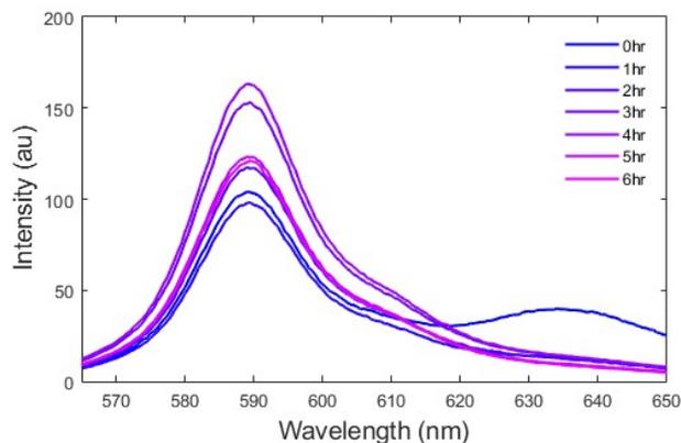
Figure S6: Fluorescence emission spectra for acetone-based solution containing resazurin and 1% v/v H<sub>2</sub>O after exposure to iron. The distinctive, but low intensity single peak attributed to resorufin can be seen after 0 hr indicates a reduction of resazurin to resorufin, followed by the further reduction of resorufin to dihydroresorufin. The reduction from resorufin to dihydroresorufin is reversible, resulting in a small concentration of resorufin remaining in the solution.
