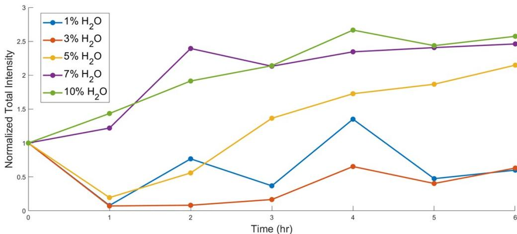
Figure S7: Normalized integrated fluorescence intensity over time for DMSO-based solutions containing 50  $\mu$ M resazurin and 1%, 3%, 5%, 7%, and 10% H<sub>2</sub>O by volume after being introduced to iron. Because of supply chain issues and the fast degradation rate of DMSO upon exposure to air we have been unable to collect replicate data.
