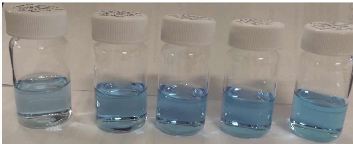
Figure S14: Acetone-based solutions containing resazurin before the addition of iron. From left to right, 1%, 3%, 5%, 7%, and 10% H<sub>2</sub>O by volume.
