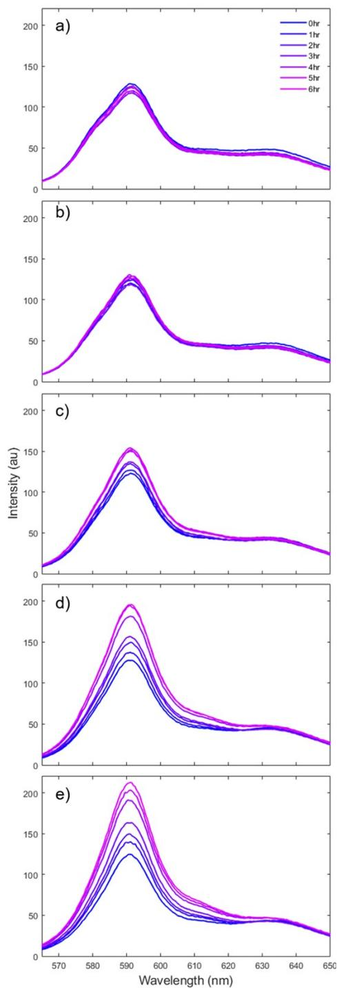
Figure S8: Fluorescence emission spectra for ethanol-based solutions containing resazurin and a) 1%, b) 3%, c) 5%, d) 7%, and e) 10% H<sub>2</sub>O by volume after being introduced to iron.
