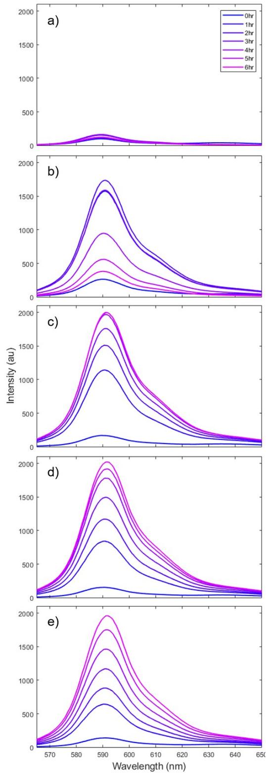
Figure S12: Fluorescence emission spectra for acetone-based solutions containing resazurin and a) 1%, b) 3%, c) 5%, d) 7%, and e) 10% H<sub>2</sub>O by volume after being introduced to iron.
