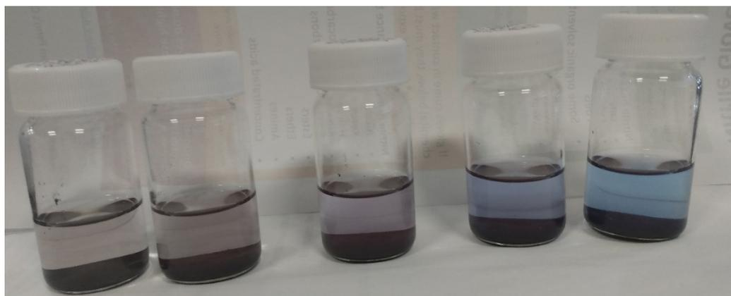
Figure S5: Acetone-based solutions containing resazurin 30 minutes after the addition of iron. From left to right, 1%, 3%, 5%, 7%, and 10% H<sub>2</sub>O by volume. A shift in solution color from blue to pink occurs as resazurin is reduced to resorufin. A shift in solution color from pink to clear occurs as resorufin is further reduced to dihydroresorufin.
