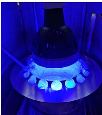
**Figure S1. Temperature controlled reaction setup (35 W blue LED)**
