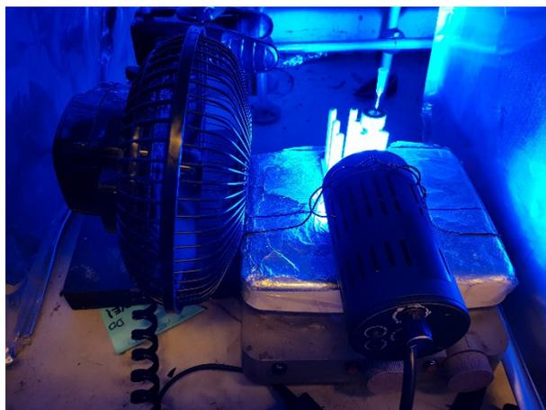
**Figure S13.** The setup for the photochemical oxygenation of arenes and alkanes under irradiation with one Kessil A160WE blue LED lamp.
