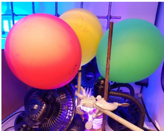
**Figure S15.** The setup for photochemical oxygenation of CH<sub>4</sub> and C<sub>2</sub>H<sub>6</sub> under one Kessil PR160-390 LED lamp and four 24 W (100 W equivalent) CFL UVA light bulbs.
