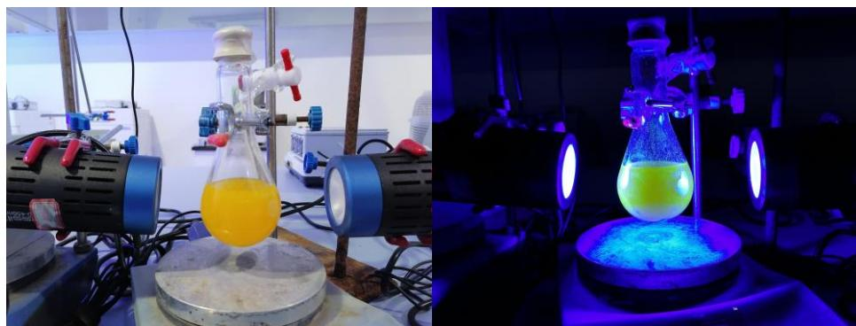
**Figure S3. Set-up of the reaction (5 mmol scale)**
