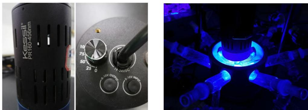
**Figure S1. Light source and photoreactor used in this research**
