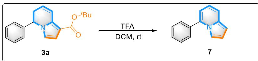
Synthesis method: A solution of indolizine **3a** (58.6 mg, 0.2 mmol) and TFA (15 μL, 0.2 mmol) in DCM (2 mL) was stirred at rt for 19 h. After the reaction was complete, the reaction mixture was concentrated to give the crude. The crude product was purified by flash column chromatography on silica gel (EtOAc/Petroleum = 50/1) to obtain the desired compound **7** as a dark green oil (18.5 mg, 48%).
