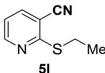
Yellow oil, 21.3 mg, yield: 65% (known compound<sup>11</sup>). <sup>1</sup>H NMR (300 MHz, CDCl<sub>3</sub>) δ 8.52 – 8.49 (m, 1H), 7.73 – 7.70 (m, 1H), 7.01 – 6.97 (m, 1H), 3.20 (q, *J* = 7.4 Hz, 2H), 1.33 (t, *J* = 7.3 Hz, 3H). <sup>13</sup>C NMR (75 MHz, CDCl<sub>3</sub>) δ 162.28, 151.08, 139.49, 117.30, 114.58, 106.41, 23.66, 13.32.
