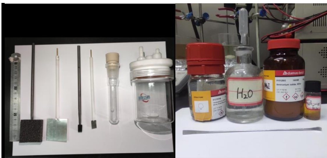
Figure S5: ( Left ): General equipment for electrolysis. ( Right ): All reagents for this reaction.
