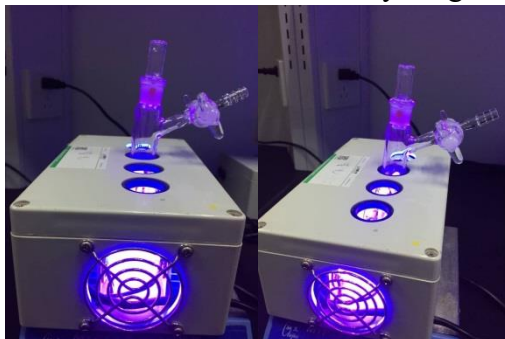
Figure S1. Photoreactor used in this research (2 x 3 W purple LEDs, \lambda_{\text{max}} = 398 nm)
