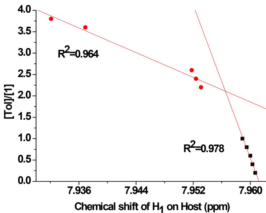
Figure S15. Mole ratio plot of the complexation of **1** and Tol in CDCl<sub>3</sub> at 298 K.
