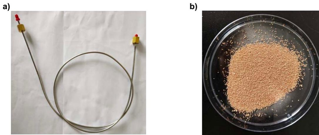
**Figure S7.** (a) photo of host **1** packed column. (b) red carrier 6201 that loaded 5% wt host **1**.
