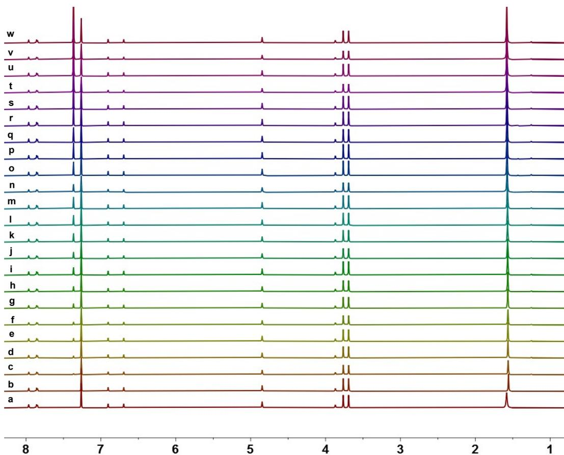
**Figure S8.**  $^1\text{H}$  NMR spectra (400 MHz,  $\text{CDCl}_3$ , v/v, 298 K) of **1** at a concentration of 1.0 mM with different concentrations of **PhH**: (a) 0.00 mM; (b) 0.2 mM; (c) 0.4 mM; (d) 0.6 mM; (e) 0.8 mM; (f) 1.0 mM; (g) 1.2 mM; (h) 1.4 mM; (i) 1.6mM; (j) 1.8 mM; (k) 2.0 mM; (l) 2.2 mM; (m) 2.4 mM; (n) 2.6 mM; (o) 2.8 mM; (p)3.0 mM; (q) 3.2 mM; (r) 4.0 mM; (s) 6.0 mM; (t) 8.0 mM; (u) 10.0 mM; (v) 30.0 mM; (w) 50.0 mM.
