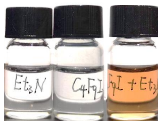
Figure S3. Photograph of solution of \text{Et}_3\text{N} , \text{C}_4\text{F}_9\text{I} and mixture solution of \text{Et}_3\text{N}/\text{C}_4\text{F}_9\text{I} in \text{DMSO} / \text{CH}_3\text{OH} (99:1, v/v) ( c = 0.01 \text{ M} ).
