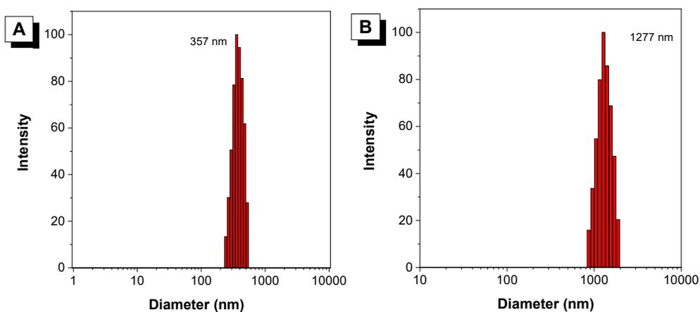
**Figure S28.** Dynamic light scattering diagram of Boc-*D*-Alanine + *R*-7 (A) and Boc-*L*-Alanine + *R*-7 (B) in DMF/H<sub>2</sub>O (60/40), respectively.
