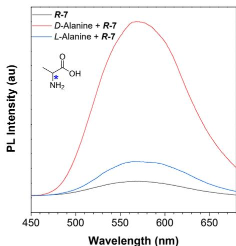
**Figure S18** PL spectra of a mixture of *R-7* and enantiomers of Alanine in DMSO/H<sub>2</sub>O (v/v, 3/2).  $[R-7] = 1/2[\text{analyte}] = 1.0 \times 10^{-5} \text{ M}$ ,  $\lambda_{\text{ex}} = 369 \text{ nm}$ .  $I_D/I_L = 4.86$ .
