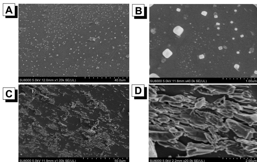
**Figure S27.** SEM images of the mixture (A and B: *D-Boc-Alanine* + *R-7*, C and D: *L-Boc-Alanine* + *R-7*) in DMF/Water (v/v, 60/40),  $[R-7] = 1.0 \times 10^{-5}$  M.
