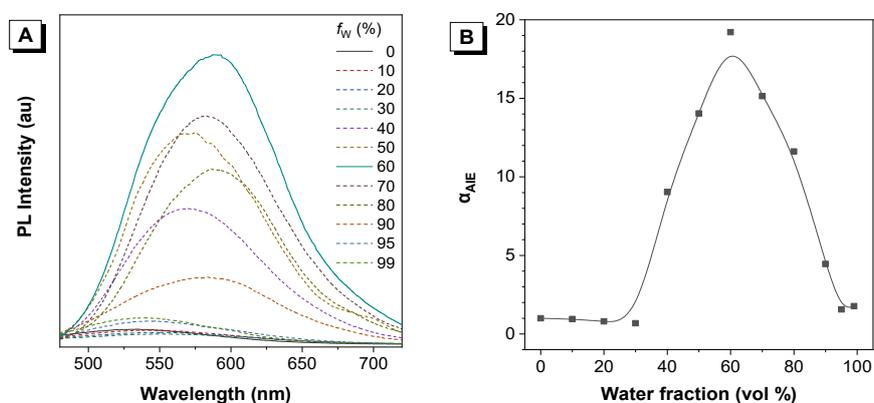
**Figure S13.** (A) PL spectra of *R-7* in DMF/water mixture with different water fraction. Excitation wavelength: 369 nm,  $[R-7] = 1.0 \times 10^{-5}$  M. (B) Fluorescence intensity ratio of  $\alpha_{AIE}$  in different DMF/water mixture.
