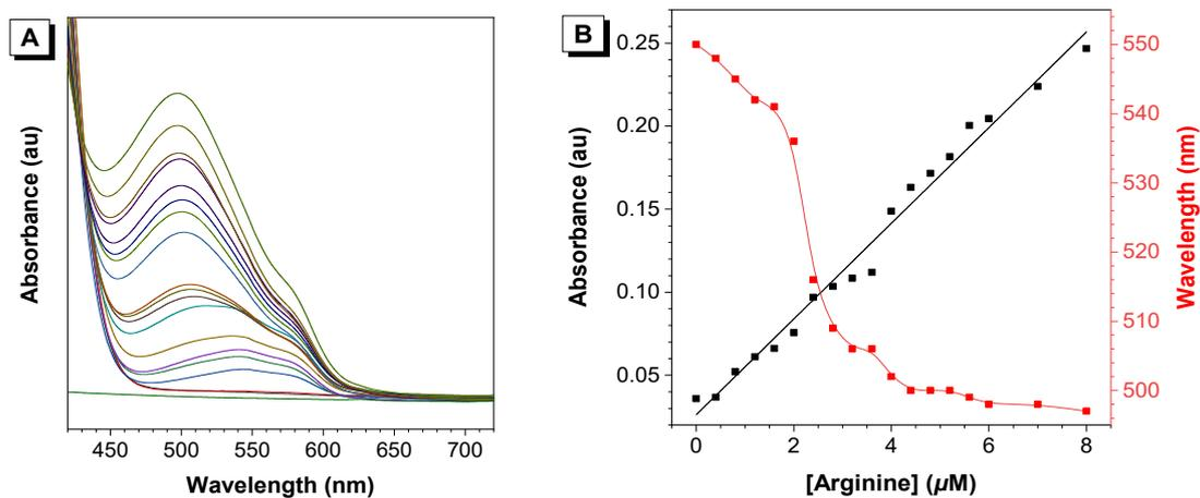
**Figure S36.** (A) The absorbance curve of Arginine at  $0 \times 10^{-6}$  M to  $8 \times 10^{-5}$  M + **R-7** ( $2 \times 10^{-5}$  M), in DMSO. (B) Plot of absorbance intensity in different concentrations. According to  $\text{LOD} = 3\delta/s^2$ , the limit of detection is  $2.38 \times 10^{-7}$  M.
