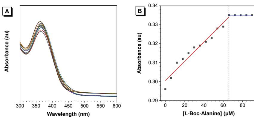
**Figure S16.** (A) UV-vis titration of *R-7* ( $1.0 \times 10^{-5}$  M) in the presence of 0 to 90  $\mu\text{M}$  of *L*-Boc-Alanine in DMF/H<sub>2</sub>O (60/40). (B) Curve of absorbance versus concentration of *L*-Boc-Alanine. [*R-7*] = 30  $\mu\text{M}$ .
