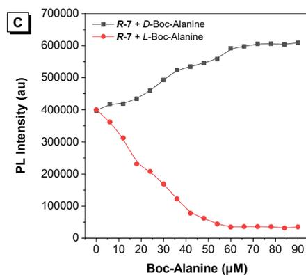
**Figure S15.** (A) PL titration of *R-7* ( $1.0 \times 10^{-5}$  M) in the presence of 0 to 90  $\mu\text{M}$  of *D*-Boc-Alanine in DMF/H<sub>2</sub>O (60/40); (B) PL titration of *R-7* in the presence of 0 to 90  $\mu\text{M}$  of *L*-Boc-Alanine in DMF/H<sub>2</sub>O (60/40); (C) Curve of PL intensity versus concentration of Boc-Alanine.
