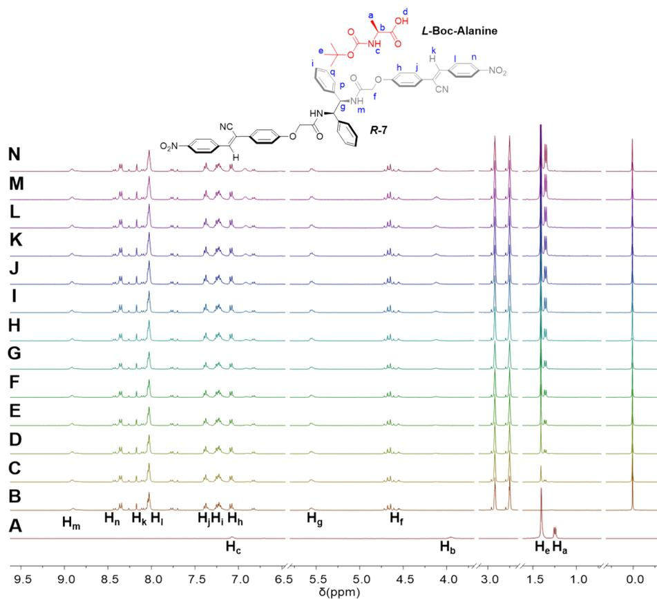
**Figure S21.**  $^1\text{H}$  NMR titration of the *R-7* and *L*-Boc-alanine system in  $\text{DMF-}d_7$  at 298 K. (A) Resonance signals for the free *L*-Boc-alanine (4.0 mM). (B) Resonance signals for the free *R-7* (4.0 mM). (C–N) Changes in resonance signals of *L*-Boc-alanine in the presence of 0.2 to 3.0 equivalents of *R-7*.
