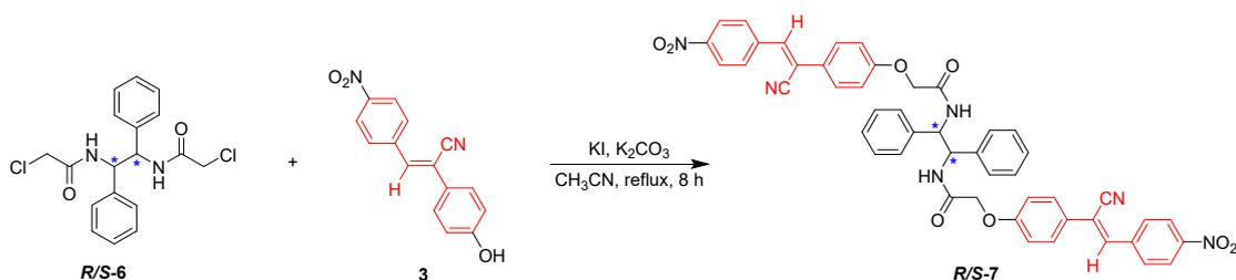
**Scheme S3.** Synthetic procedure of chiral AIEgens **R-7** and **S-7**.
