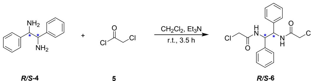
**Scheme S2.** Synthetic procedure of chiral compound *R/S*-6.
