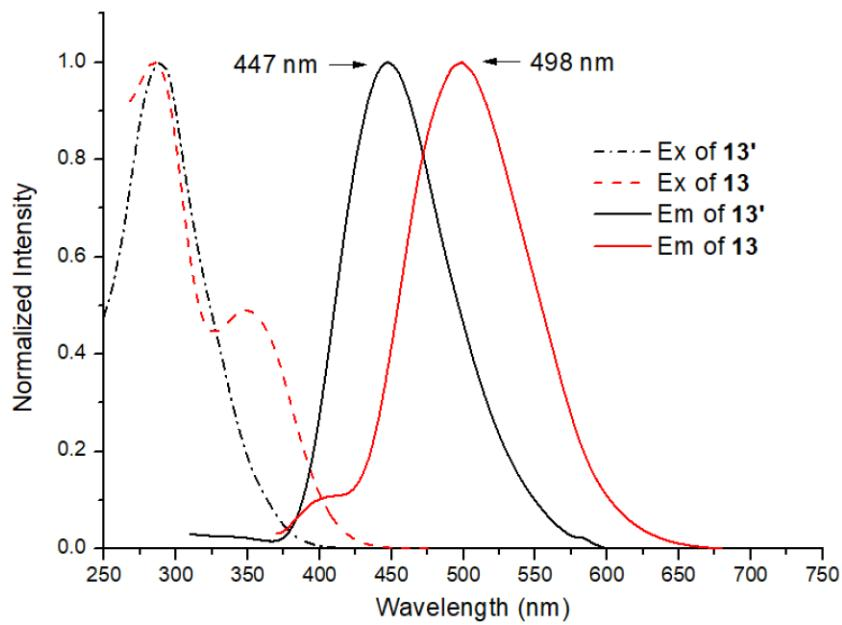
**Figure S3** (Dashed line) excitation spectra and (full line) emission spectra of **13** and **13'**. (**13**:  $\lambda_{\text{ex}} = 290 \text{ nm}$ ; **13'**:  $\lambda_{\text{ex}} = 350 \text{ nm}$ ).
