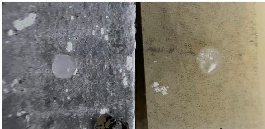
Fig. S7. The anti-icing performance. The droplets freeze on the hollow sphere surface and PVC surface is 5.1 min and 0.2 min, respectively.
