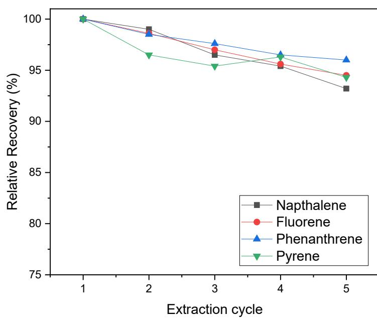
**Figure S9.** Results of the reusability study of the sol-gel C<sub>18</sub> coated FPSE media
