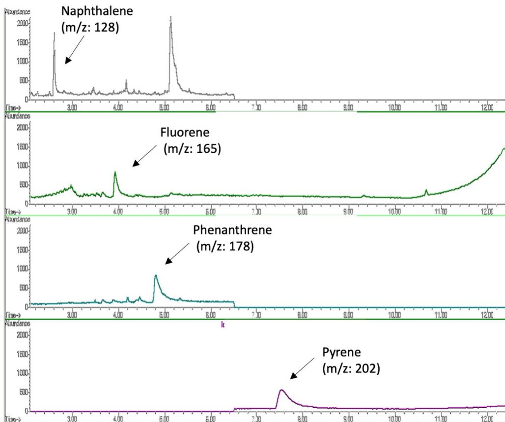
**Figure S2.** Representative chromatogram of a spiked herbal infusion sample ( $c= 10.00 \text{ ng mL}^{-1}$ )
