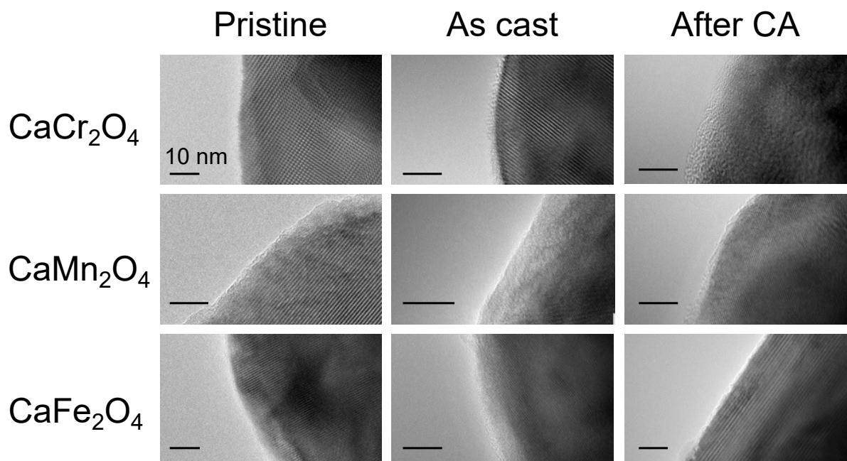
**Fig. S3** HRTEM images of postspinel oxides,  $\text{CaCr}_2\text{O}_4$ ,  $\text{CaMn}_2\text{O}_4$ , and  $\text{CaFe}_2\text{O}_4$  in pristine (left), as-cast (middle), after chronoamperometry (right) at 1.6 V vs. RHE for 1h. The bars show 10 nm.
