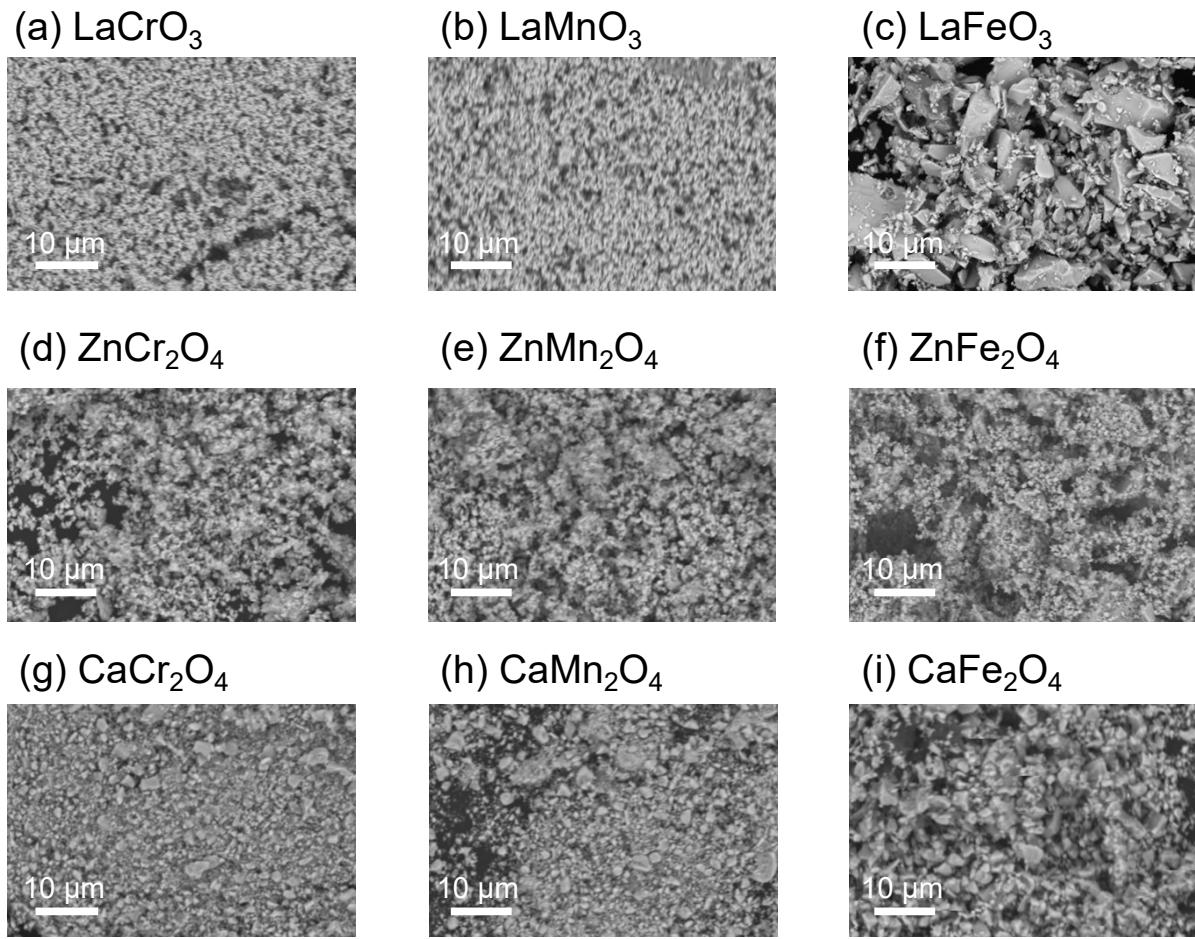
**Fig. S2** SEM images for perovskite oxides: (a) LaCrO<sub>3</sub>, (b) LaMnO<sub>3</sub>, and (c) LaFeO<sub>3</sub>, spinel oxides: (a) ZnCr<sub>2</sub>O<sub>4</sub>, (b) ZnMn<sub>2</sub>O<sub>4</sub>, and (c) ZnFe<sub>2</sub>O<sub>4</sub>, and postspinel oxides: (d) CaCr<sub>2</sub>O<sub>4</sub>, (e) CaMn<sub>2</sub>O<sub>4</sub>, and (f) CaFe<sub>2</sub>O<sub>4</sub>.
