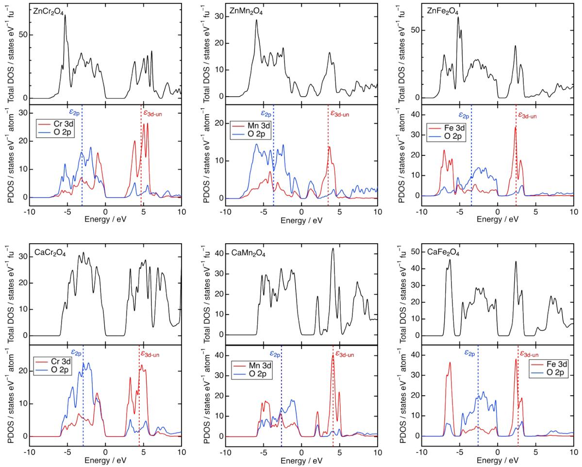
**Fig. S4** Total density of states (DOS) and partial DOS (PDOS) for  $\text{ZnB}_2\text{O}_4$  and  $\text{CaB}_2\text{O}_4$  ( $B = \text{Cr, Mn, Fe}$ ) obtained by DFT calculation.
