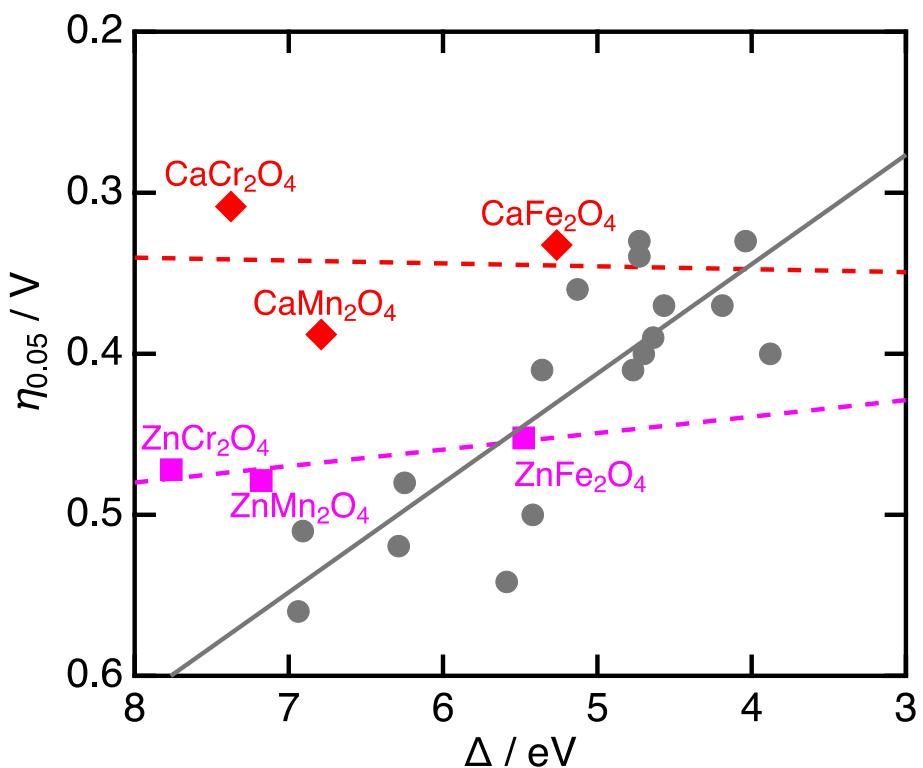
**Fig. S5** Overpotential as a function of charge-transfer energy ( $\Delta$ ) for ZnB<sub>2</sub>O<sub>4</sub>, LaBO<sub>3</sub>, and CaB<sub>2</sub>O<sub>4</sub>. The data for perovskite oxides were taken from the reference.<sup>1,2</sup> The lines were obtained from linear fitting.
