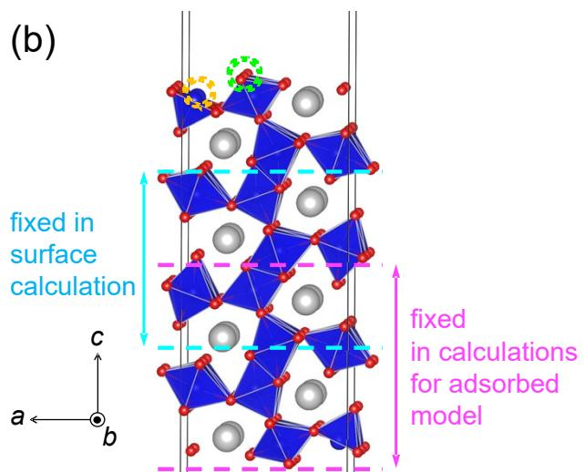
**Fig. S6** Schematics for slab models for  $\text{CaFe}_2\text{O}_4$  (001) plane. Top views are illustrated in (a).
