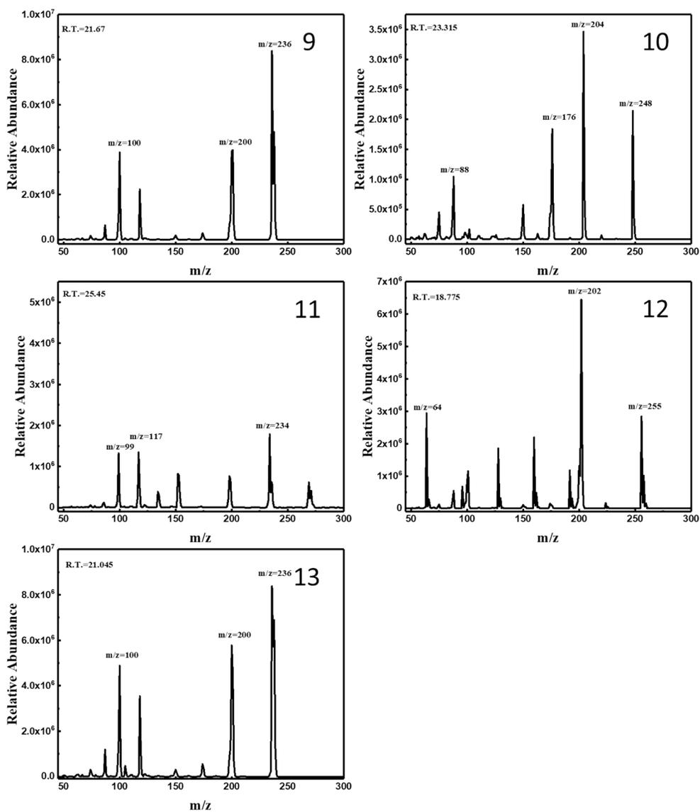
Fig. S4 Mass spectra of anthracene, phenanthrene, pyrene, fluoranthene and their degradation intermediates by HOCl oxidation. R.T.=retention time. Experimental conditions: [PAHs]<sub>0</sub> = 1 mg/L, [Cl<sub>2</sub>]<sub>0</sub> = 100 mg/L, pH = 5, reaction time = 12 h.
