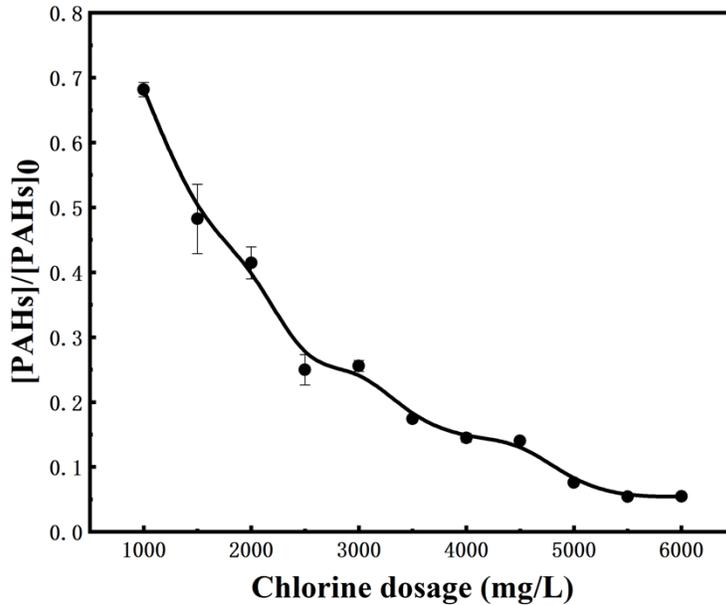
Fig. S1. The degradation of PAHs with different effective chlorine dosages.
