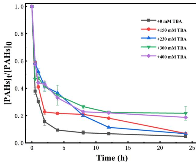
Fig.S2. The effect of TBA dosages on the PAHs degradation in the contaminated industrial soil by HOCl oxidation. Experimental conditions:  $[\text{PAHs}]_0=2469.9$  mg/kg,  $[\text{Cl}_2]_0=5000$  mg/L, pH=5.
