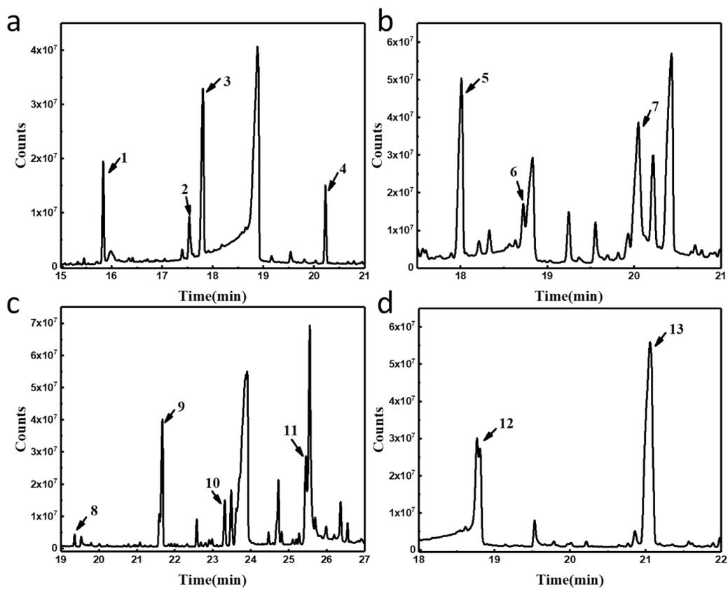
Fig.S3 Total ion chromatogram of degradation products by HOCl oxidation of (a) anthracene, (b) phenanthrene, (c) pyrene, and (d) fluoranthene. Experimental conditions:  $[\text{PAHs}]_0 = 1 \text{ mg/L}$ ,  $[\text{Cl}_2]_0 = 100 \text{ mg/L}$ ,  $\text{pH} = 5$ , reaction time = 12 h.
