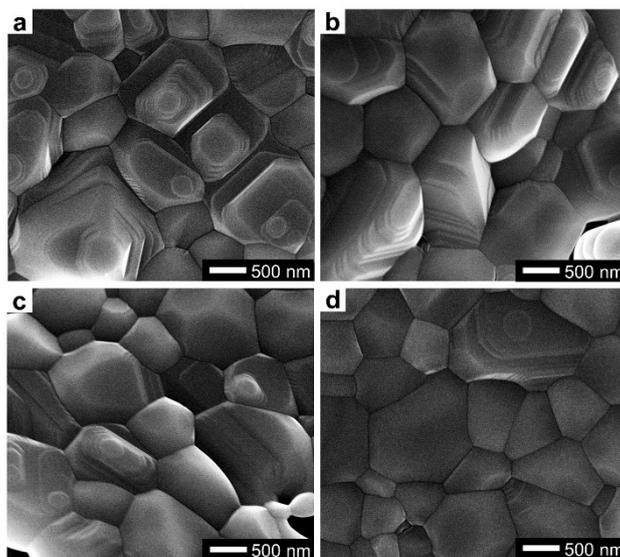
**Fig. S4** High magnification SEM images of different HA dish samples: (a) Meso-1; (b) Meso-2; (c) Meso-3; (d) Meso-4.
