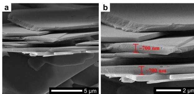
**Fig. S1** SEM images of  $\text{CaHPO}_4$  particles in cross-section view. (a) Low magnification. (b) High magnification.
