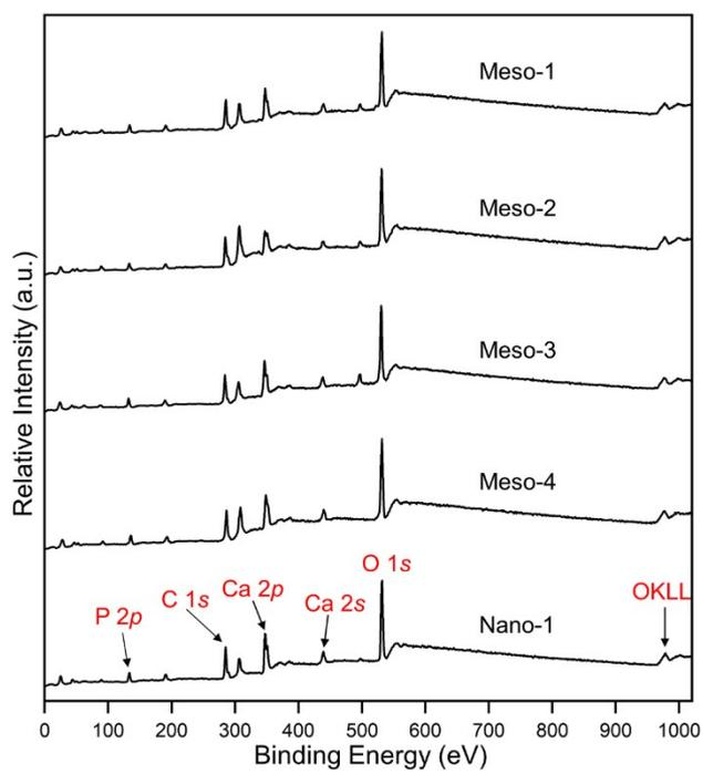
**Fig. S12** XPS full spectra of different HA dish samples.
