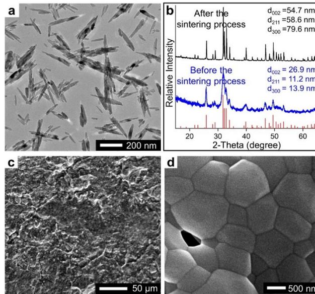
**Fig. S2** (a) TEM image of HA nanoparticles. (b) XRD patterns of the HA nanoparticles and the Nano-1 dishes. (c) and (d) SEM images of Nano-1 dishes.
