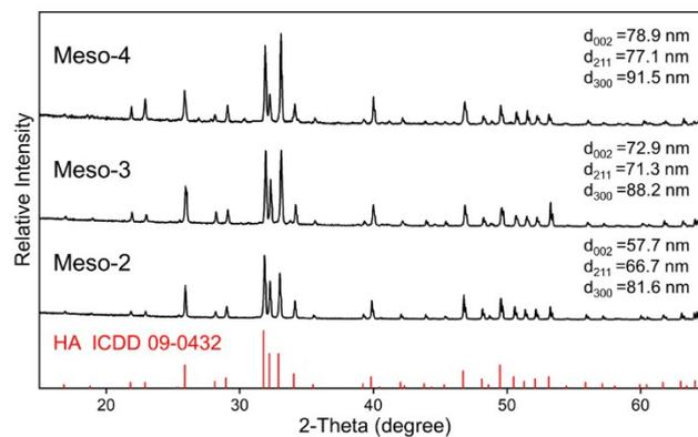
**Fig. S5** XRD patterns of different HA dish samples.
