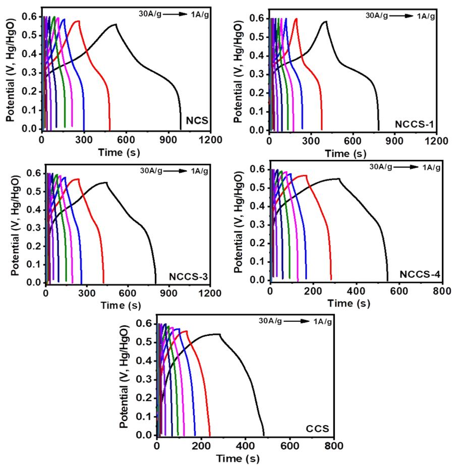
**Figure S7.** GCD curves of NCS, NCCS-1, NCCS-3, NCCS-4, and CCS at various current densities of 1-30 A/g in KOH.
