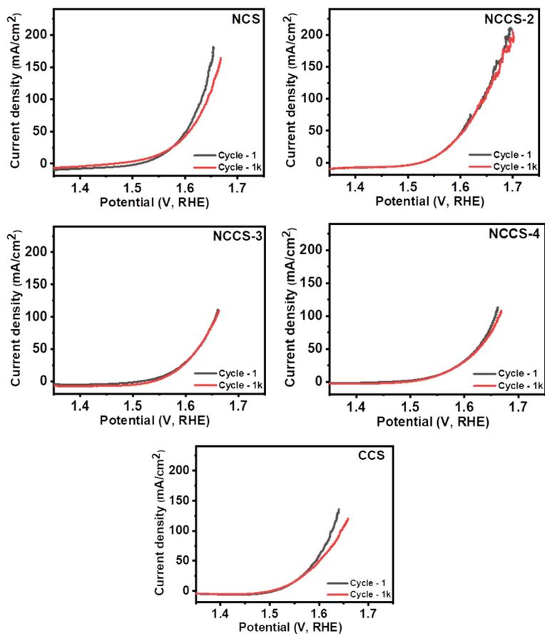
**Figure S10.** 1<sup>st</sup> and 1k cycle OER polarization curves for NCS, NCCS-2, NCCS-3, NCCS-4, and CCS in KOH.
