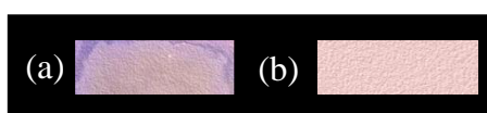
Fig. S13 (a) The fluorescent test paper without Nafion solution + 30 μM NO 2 - under UV light; (b) The fluorescent test paper with Nafion solution + 30 μM NO 2 - under UV light.
