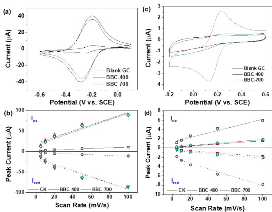
Figure S5 (a, b) CV scans of the blank glassy carbon electrode (blank GC) and GC loaded with BBC-400 and BBC-700 at scan rate of 20 mV/s in PBS with 0.5 mM hexaammineruthenium(III) chloride or 0.5 mM potassium ferricyanide; (c, d) the peak current of oxidation or reduction for reversible redox reactions of  $\text{Ru}^{3+}$  (positive ion) and  $[\text{Fe}(\text{CN})_6]^{3-}$  (negative ion) at various scan rates.
