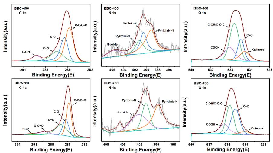
Figure S3 O 1s, C 1s and N 1s X-ray photoelectron spectroscopy (XPS) of BBC-400 (a) and BBC-700 (b), respectively.
