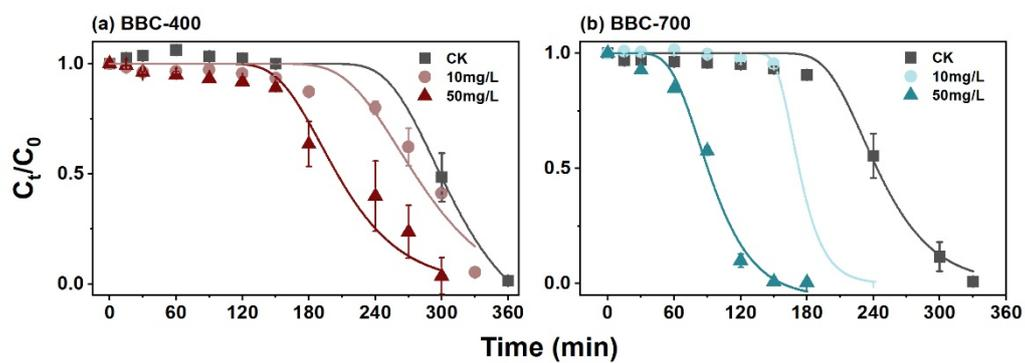
Figure S12 Methyl orange degradation by sulfide in the absence or presence of (a) BBC-400 and (b) BBC-700 with different concentrations (10mg/L and 50mg/L).
