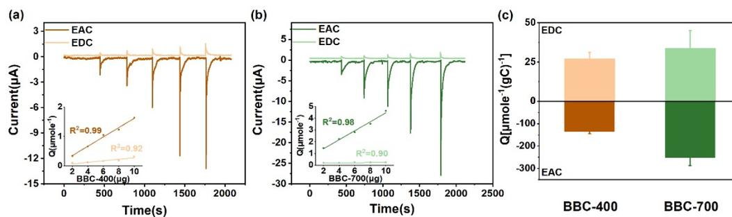
**Figure S10** (a) Reductive and oxidative current responses of BBC-400 (Inset: Linear relationship between the electron numbers and the added amounts of BBC-400); (b) reductive and oxidative current responses of BBC-700 (Inset: Linear relationship between the electron numbers and the added amounts of BBC-700); (c) electron transfer capacity of BBC-400 and BBC-700.
