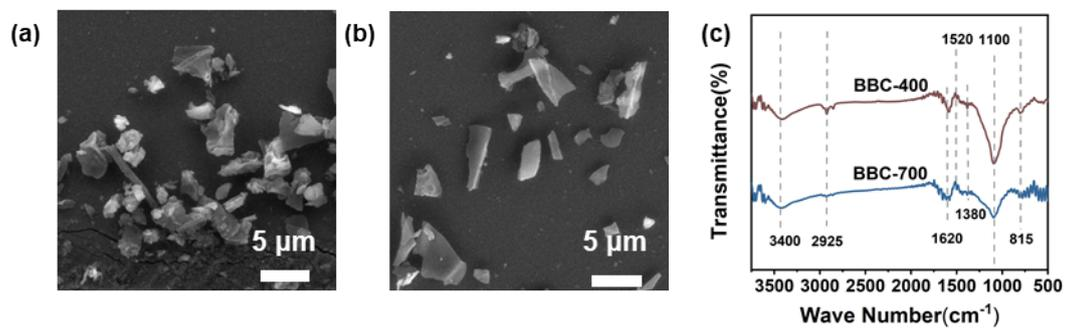
**Figure S1** (a, b) SEM images and (c) FTIR spectra of bulk-biochar-400 (BBC-400) and bulk-biochar-700 (BBC-700).
