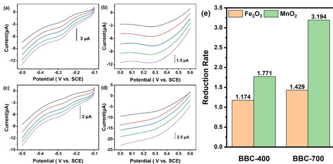
**Figure S11** Linear sweep voltammograms of hematite ( $\text{Fe}_2\text{O}_3$ ) and  $\text{MnO}_2$  on BBC-400 and BBC-700 electrode. Scan rates varied from  $50$  to  $250 \text{ mV}\cdot\text{s}^{-1}$  with an interval of  $50 \text{ mV}\cdot\text{s}^{-1}$ . and (e) the reduction rate comparison among minerals (hematite and  $\text{MnO}_2$ ) at  $200 \text{ mV}/\text{s}$  scan rate.
