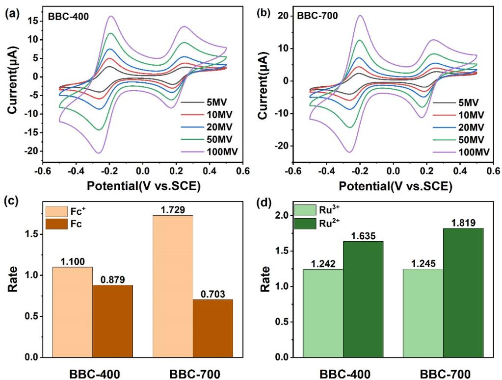
Figure S9 CV scans of (a) BBC-400 and (b) BBC-700 treatment under different scan rates (5, 10, 20, 50 and 100 mV) in PBS containing 0.5 mM  $\text{Ru}^{3+}$  and  $\text{Fc}$ . The amplification ratios (AR) of BCs in (c)  $\text{Fc}$  oxide,  $\text{Fc}^+$  reduce and (d)  $\text{Ru}^{2+}$  oxide,  $\text{Ru}^{3+}$  reduce processes at scan rate of 50 mV/s.
