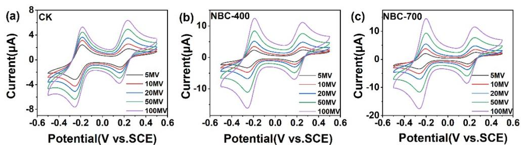
**Figure S8** (a) CV scans of CK (chitosan), (b) NBC-400 and (c) NBC-700 treatment under different scan rates (5, 10, 20, 50 and 100 mV) in PBS containing 0.5 mM  $\text{Ru}^{3+}$  and Fc.
