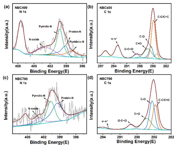
Figure S2 N 1s and C 1s X-ray photoelectron spectroscopy (XPS) of NBC-400 (a, b) and NBC-700
