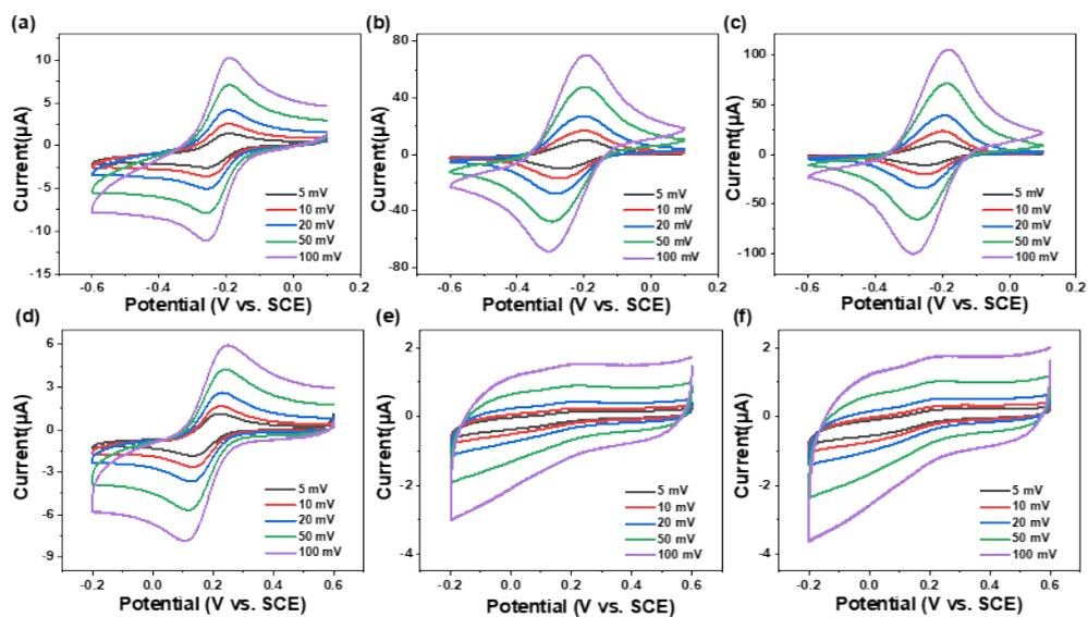
**Figure S6** CVs of blank GC, NBC-400 and NBC-700 under different scan rates (5, 10, 20, 50 and  $100 \text{ mV}\cdot\text{s}^{-1}$ ) in 0.5 mM (a, b, c) hexaammineruthenium(III) chloride solution or (d, e, f) potassium ferricyanide solution.
