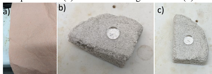
Figure S1. Hydrophobic coating adhesion test. (a) rugged paper used to rub the composite, (b) composite with water droplet before, (c) composite with water droplet after rubbing with cloth.
